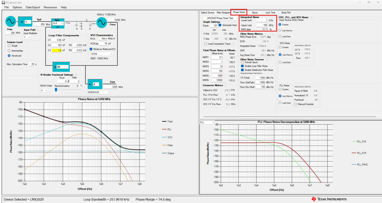
Figure 10-3. Using PLLatinum Sim to Determine Clock Jitter Across Integration Bandwidth of the Application
