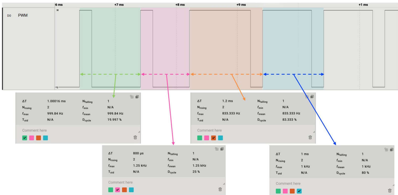
Figure 3-1. Probe PWM Changes During Updating CMPA Register in Up Count Mode
