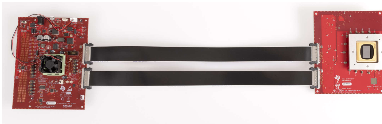
Figure 2-3. Standalone DLPLCRC964EVM and DLPLCR99EVM / DLPLCR99UVEVM
