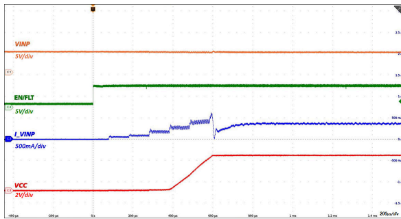
Figure 8-3. Start-Up with EN/FLT From Low to High: VINP = 5.0V, VCC = 3.3V, 11Ω Load
