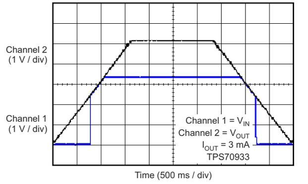
**Figure 6-34. Power-Up and Power-Down Response**
