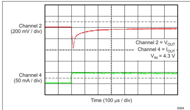
**Figure 6-25. TPS70933 Load Transient (0 mA to 50 mA)**
