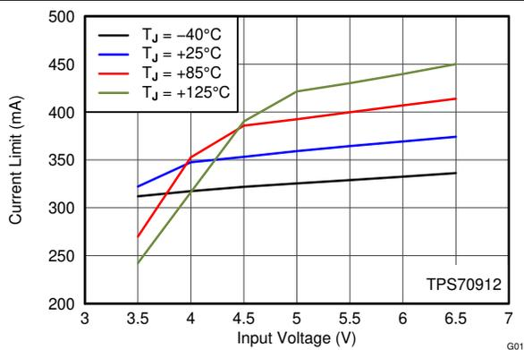
Figure 6-11. 1.2-V Current Limit vs  $V_{IN}$  and Temperature
