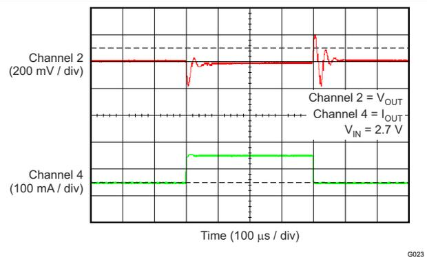
Figure 6-24. TPS70912 Load Transient (50 mA to 150 mA)
