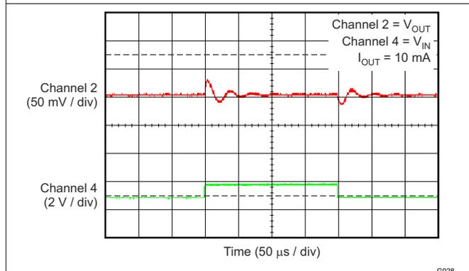
**Figure 6-29. TPS70912 Line Transient (2.7 V to 3.7 V)**
