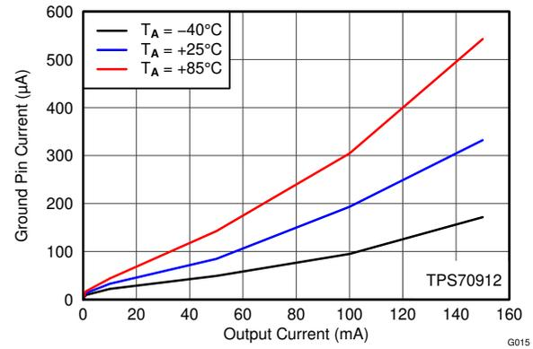
**Figure 6-16. GND Current vs  $I_{OUT}$  and Temperature**
