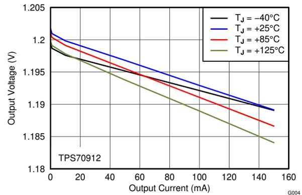
Figure 6-4. 1.2-V Load Regulation vs  $I_{OUT}$  and Temperature
