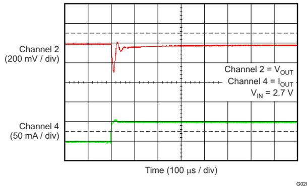
Figure 6-21. TPS70912 Load Transient (0 mA to 50 mA)
