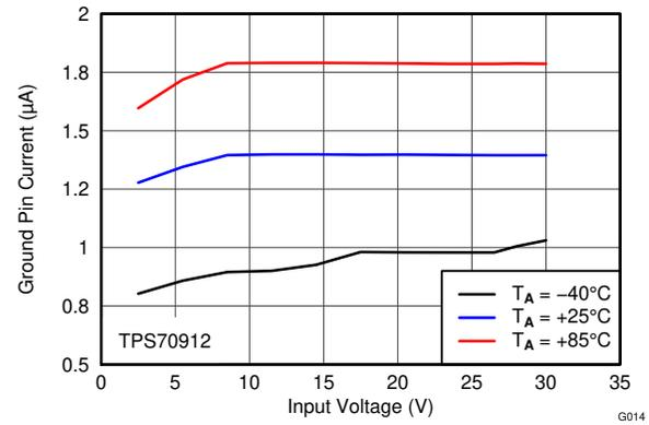
**Figure 6-14. GND Current vs  $V_{IN}$  and Temperature**
