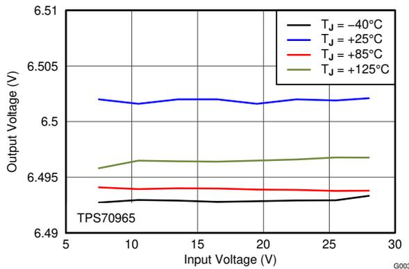
Figure 6-3. 6.5-V Line Regulation vs  $V_{IN}$  and Temperature
