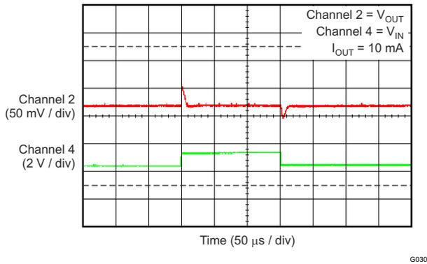
**Figure 6-31. TPS70933 Line Transient (4.3 V to 5.3 V)**
