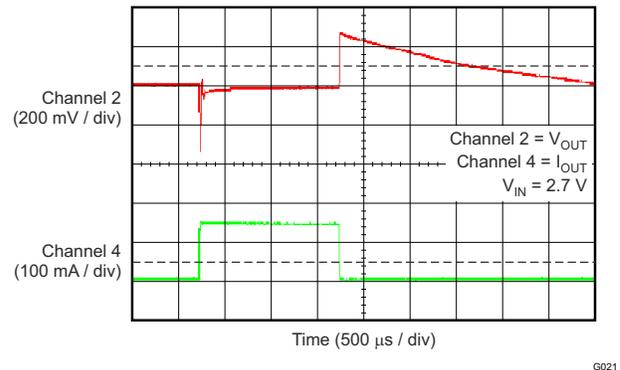
Figure 6-22. TPS70912 Load Transient (1 mA to 150 mA)
