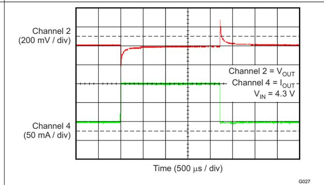
**Figure 6-28. TPS70933 Load Transient (50 mA to 150 mA)**
