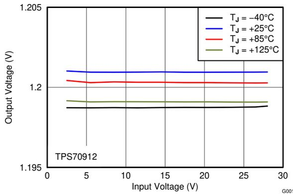
Figure 6-1. 1.2-V Line Regulation vs  $V_{IN}$  and Temperature
