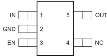
**Figure 5-1. TPS709: DBV Package, 5-Pin SOT-23, Top View**
