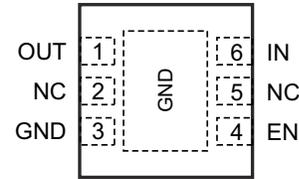
**Figure 5-4. DRV Package, 6-Pin WSON, Top View**
