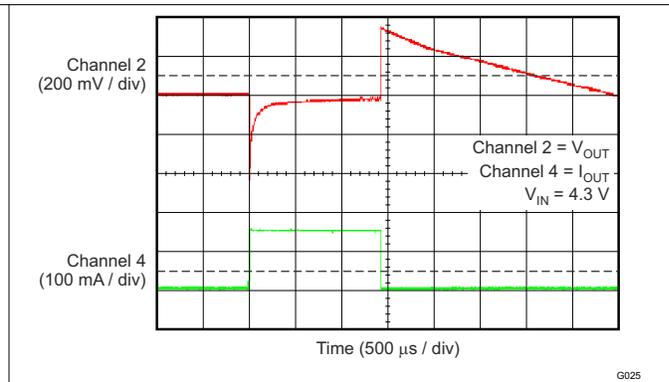
**Figure 6-26. TPS70933 Load Transient (1 mA to 150 mA)**
