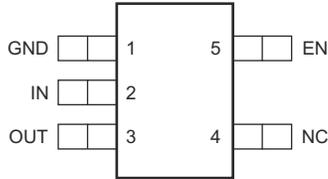
**Figure 5-3. TPS709B: DBV Package, 5-Pin SOT-23, Top View**
