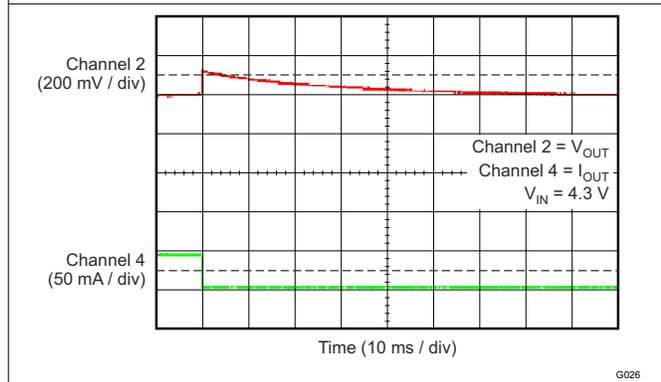
**Figure 6-27. TPS70933 Load Transient (50 mA to 0 mA)**
