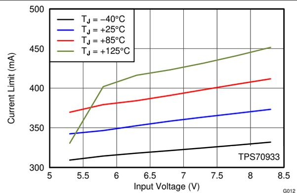
Figure 6-12. 3.3-V Current Limit vs  $V_{IN}$  and Temperature
