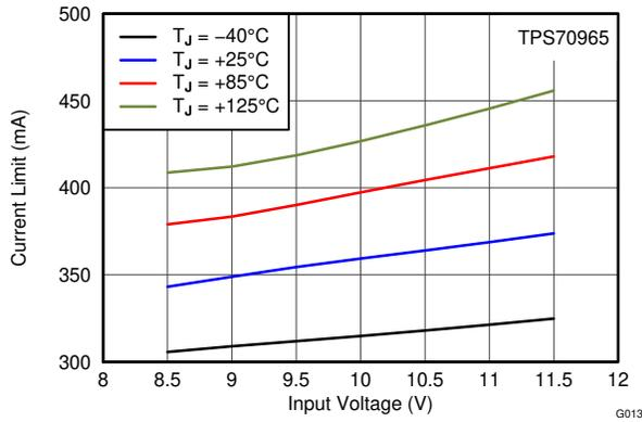
**Figure 6-13. 6.5-V Current Limit vs  $V_{IN}$  and Temperature**
