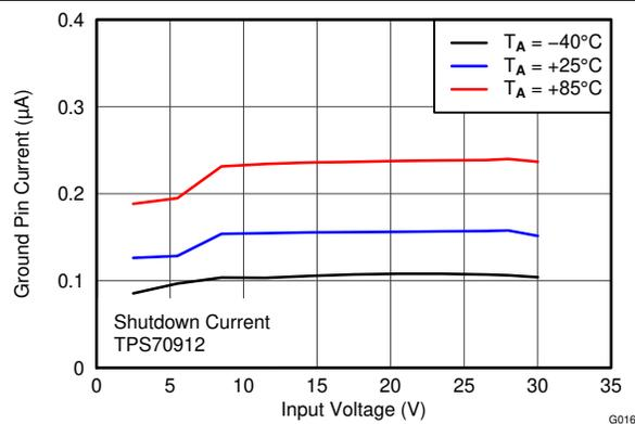
**Figure 6-17. Shutdown Current vs  $V_{IN}$  and Temperature**
