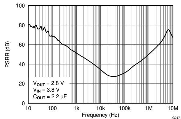
**Figure 6-18. Power-Supply Rejection Ratio vs Frequency**
