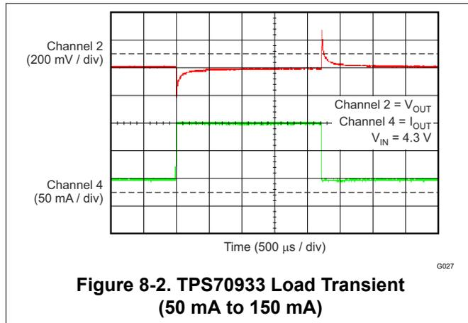
**Figure 8-2. TPS70933 Load Transient (50 mA to 150 mA)**
