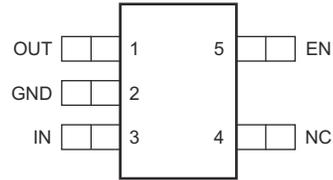
**Figure 5-2. TPS709A: DBV Package, 5-Pin SOT-23, Top View**
