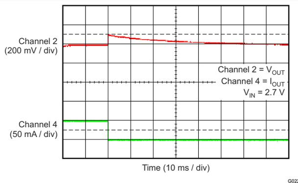
Figure 6-23. TPS70912 Load Transient (50 mA to 0 mA)
