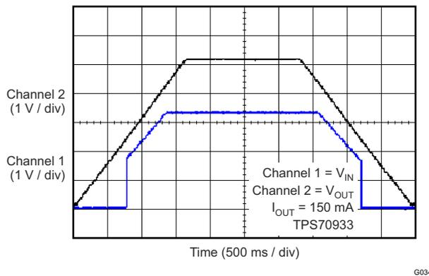
**Figure 6-35. Power-Up and Power-Down Response**
