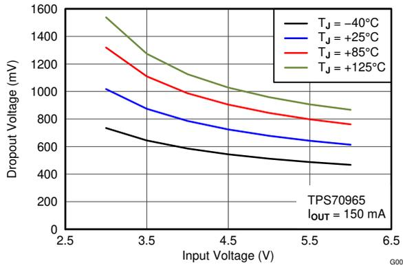
Figure 6-9. Dropout Voltage vs  $V_{IN}$  and Temperature
