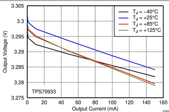
Figure 6-5. 3.3-V Load Regulation vs  $I_{OUT}$  and Temperature
