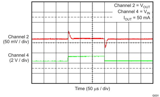
**Figure 6-32. TPS70933 Line Transient (4.3 V to 5.3 V)**
