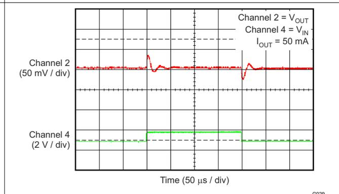
**Figure 6-30. TPS70912 Line Transient (2.7 V to 3.7 V)**
