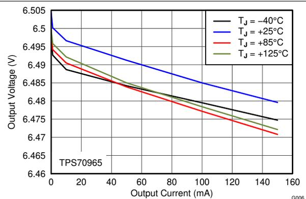
Figure 6-6. 6.5-V Load Regulation vs  $I_{OUT}$  and Temperature
