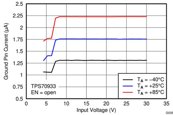
**Figure 6-15. GND Current vs  $V_{IN}$  and Temperature**
