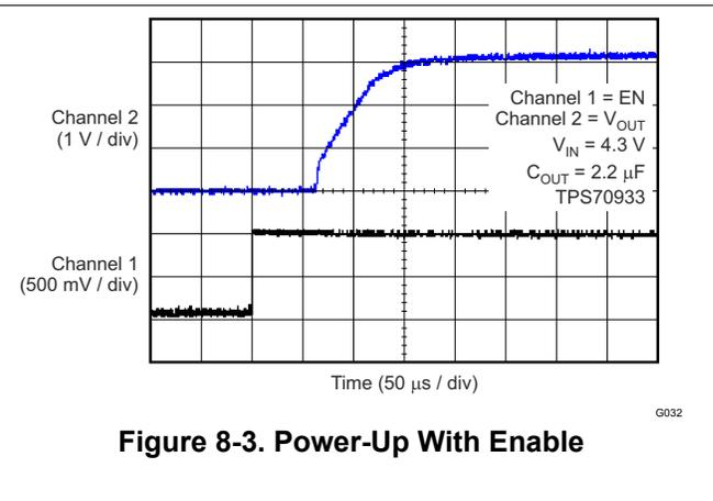
**Figure 8-3. Power-Up With Enable**
