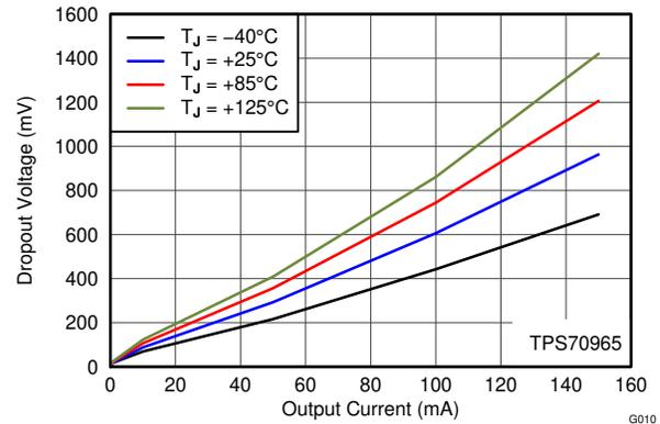
Figure 6-10. Dropout Voltage vs  $I_{OUT}$  and Temperature
