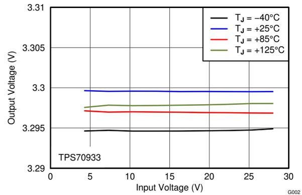
Figure 6-2. 3.3-V Line Regulation vs  $V_{IN}$  and Temperature
