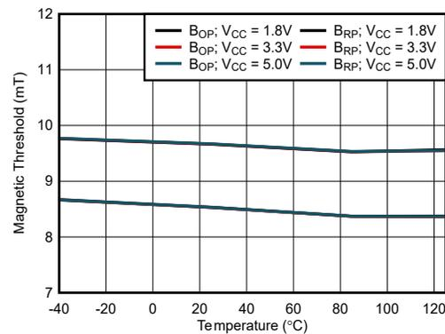
Figure 6-4. 9.5mT B<sub>OP</sub>: Thresholds vs Temperature
