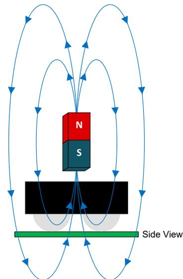
**Figure 7-4. Positive Magnetic Flux Density: Magnet In-Line**
