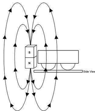
**Figure 7-3. Positive Magnetic Flux Density: Magnet Offset**
