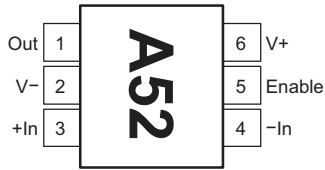
Figure 4-1. OPA300, SOT-23 Package, 6-pin (Top View)
