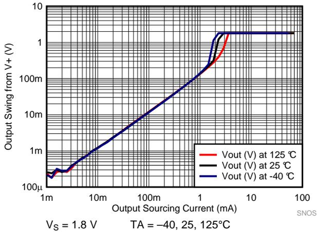
Figure 31. Output Swing vs Sourcing Current, 1.8 V
