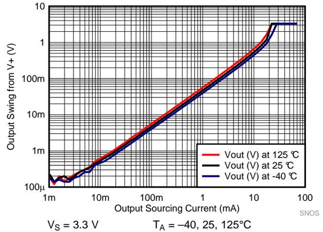
Figure 32. Output Swing vs Sourcing Current, 3.3 V
