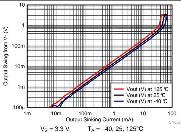
Figure 30. Output Swing vs. Sinking Current,  $3.3\text{ V}$
