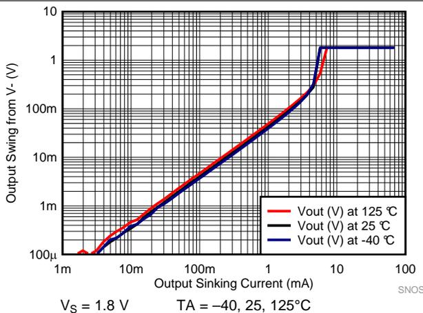
Figure 29. Output Swing vs. Sinking Current,  $1.8\text{ V}$
