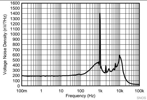
Figure 26. Voltage Noise Spectral Density vs Frequency
