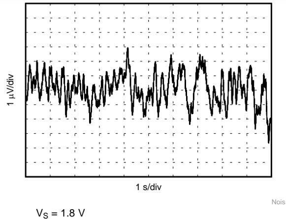
Figure 28. 0.1-Hz to 10-Hz Noise,  $V_S = 1.8\text{ V}$
