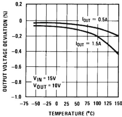
Figure 6-3. Load Regulation (New Chip)
