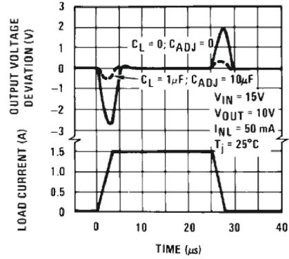
Figure 8-5. Load Transient Response (New Chip)
