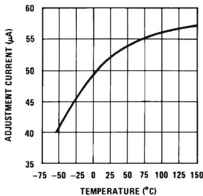
Figure 6-17. Adjustment Current vs Temperature (New Chip)
