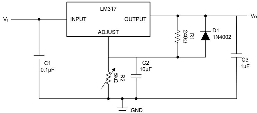
Figure 8-7. Adjustable Regulator Circuit with Improved Ripple Rejection
