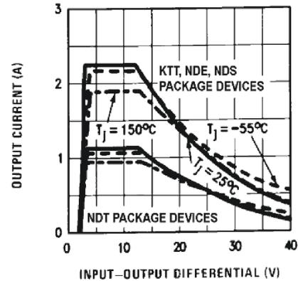
Figure 6-16. Current Limit Threshold (New Chip)
