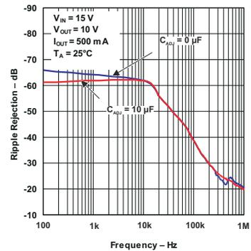
Figure 6-12. Ripple Rejection vs Frequency (Legacy Chip)
