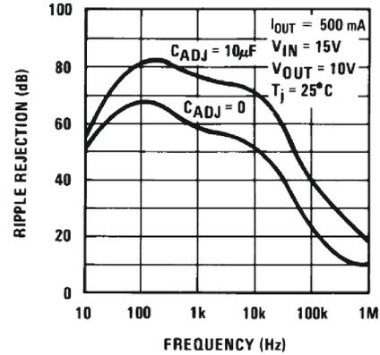
Figure 6-14. Ripple Rejection vs Frequency (New Chip)
