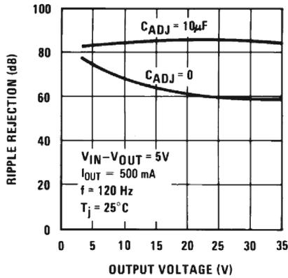
Figure 6-13. Ripple Rejection vs Output Voltage (New Chip)
