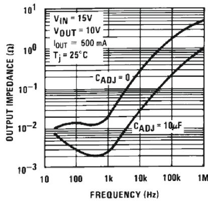
Figure 6-21. Output Impedance vs Frequency (New Chip)
