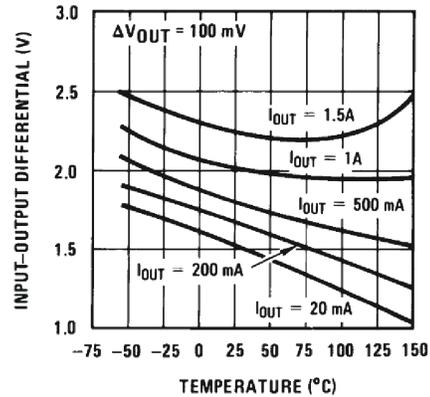
Figure 6-18. Dropout Voltage vs Temperature (New Chip)
