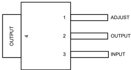
**Figure 5-1. DCY Package, 4-Pin SOT-223 (Top View)**
