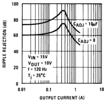
Figure 6-15. Ripple Rejection vs Output Current (New Chip)
