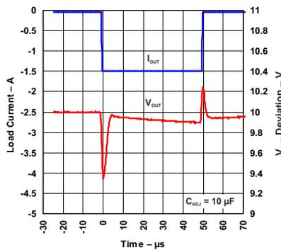
Figure 6-5. Load Transient Response (Legacy Chip)
