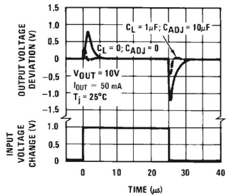
Figure 6-22. Line Transient Response (New Chip)
