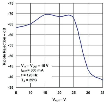
Figure 6-11. Ripple Rejection vs Output Voltage (Legacy Chip)
