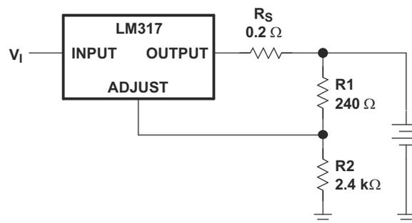
Figure 8-11. Battery-Charger Circuit
