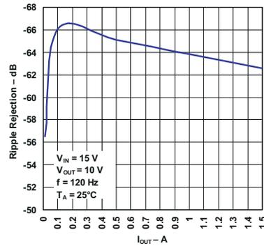
Figure 6-10. Ripple Rejection vs Output Current (Legacy Chip)
