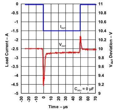
Figure 6-4. Load Transient Response (Legacy Chip)
