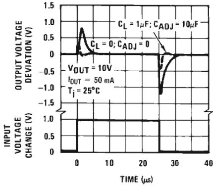
Figure 8-4. Line-Transient Response (New Chip)
