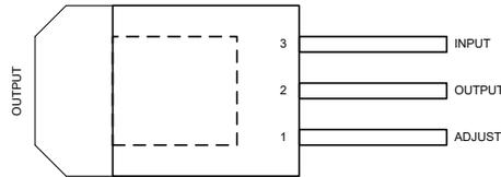
**Figure 5-3. KTT Package, 3-Pin TO-263 (Top View)**
