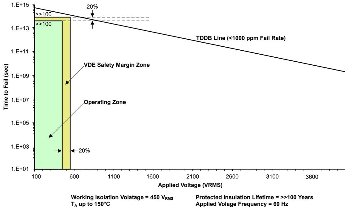
Figure 9-8. Insulation Lifetime Projection Data for 8-D Package
