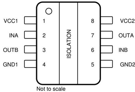
**Figure 5-3. ISO6721RB D Package 8-Pin SOIC Top View**
