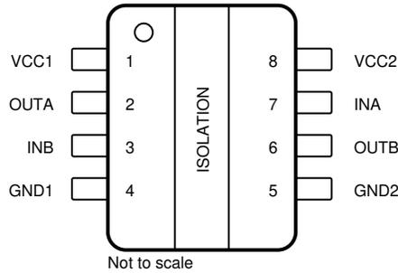
**Figure 5-2. ISO6721B D Package 8-Pin SOIC Top View**
