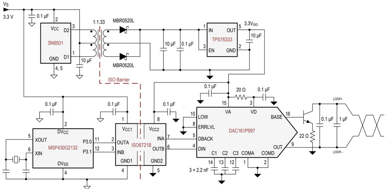
**Figure 9-1. Isolated 4-mA to 20-mA Current Loop**
