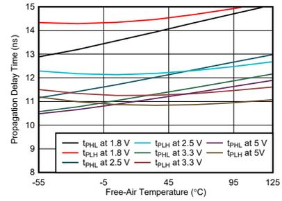
**Figure 6-14. Propagation Delay Time vs Free-Air Temperature**
