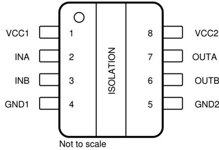
**Figure 5-1. ISO6720B D Package 8-Pin SOIC Top View**
