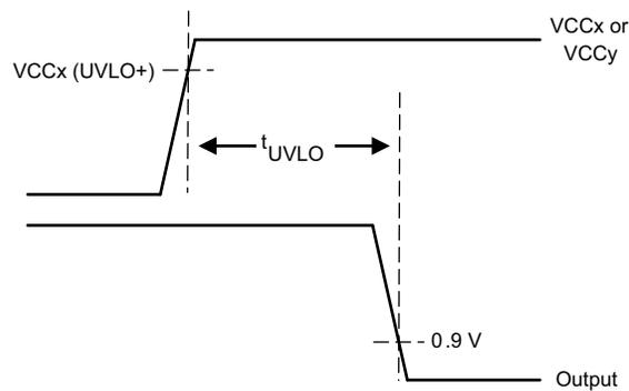
Figure 7-4.  $t_{UVLO}$  Test Circuit and Timing Diagrams
