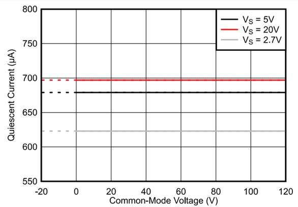
**Figure 6-38. Quiescent Current vs. Common-Mode Voltage, INA2290**
