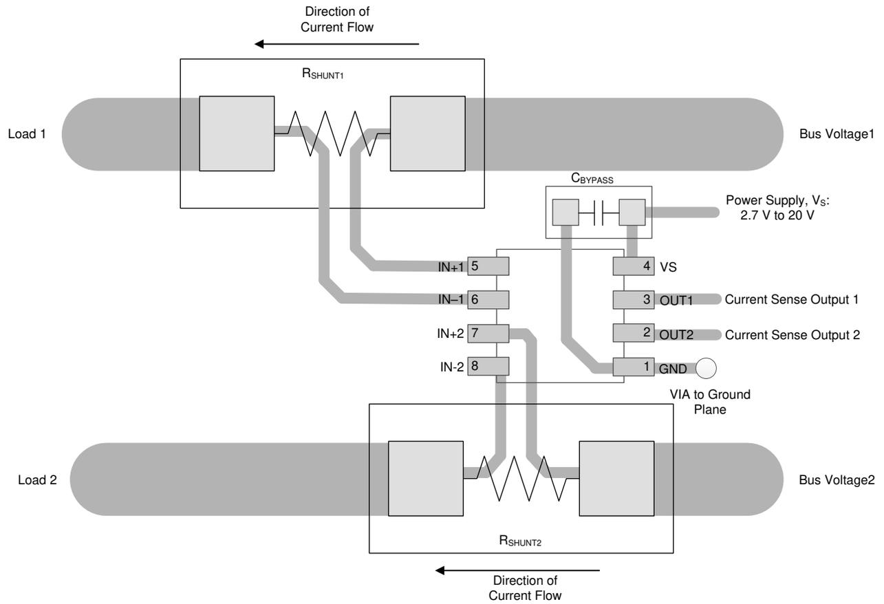
**Figure 10-2. Recommended Layout for the INA2290**
