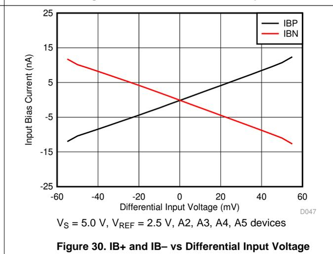
Figure 30.  $IB+$  and  $IB-$  vs Differential Input Voltage
