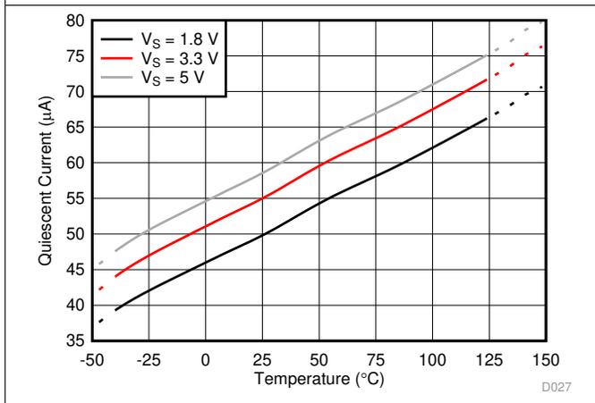
Figure 17. Quiescent Current vs Temperature (Enabled)
