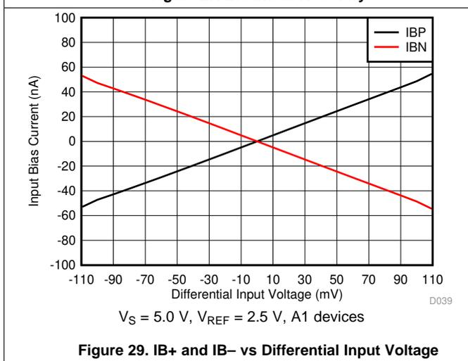
Figure 29.  $IB+$  and  $IB-$  vs Differential Input Voltage
