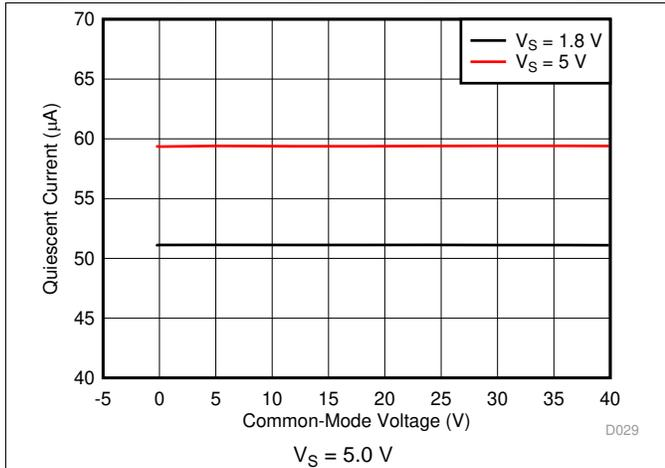
Figure 19. Quiescent Current vs Common Mode Voltage
