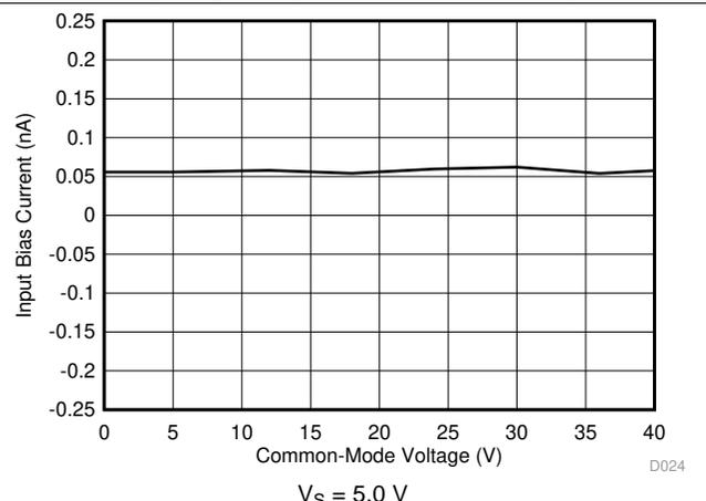
Figure 14. Input Bias Current vs Common-Mode Voltage
