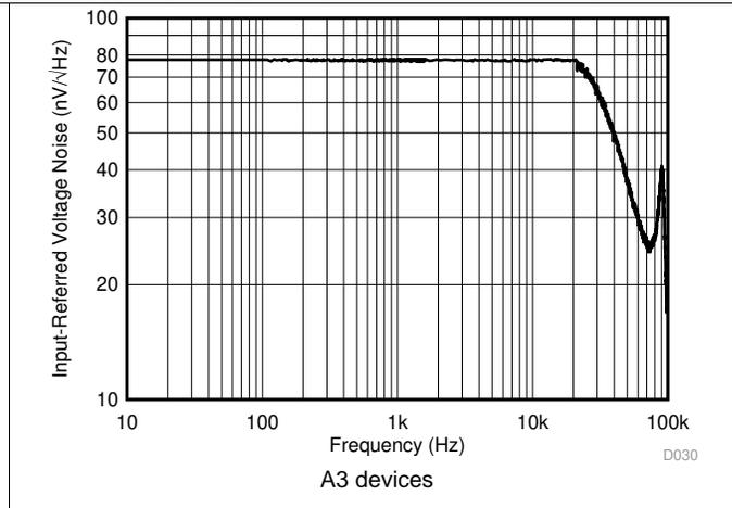
Figure 20. Input-Referred Voltage Noise vs Frequency
