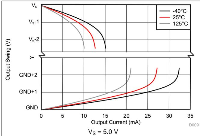
Figure 13. Output Voltage Swing vs Output Current
