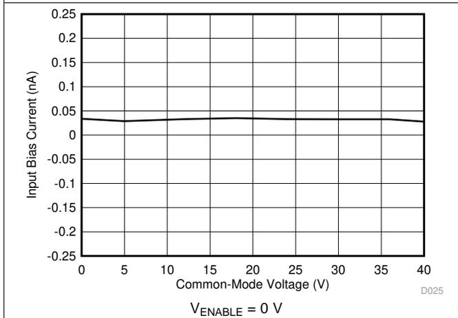
Figure 15. Input Bias Current vs Common-Mode Voltage (Shutdown)
