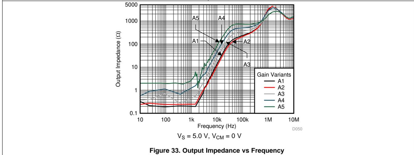
Figure 33. Output Impedance vs Frequency
