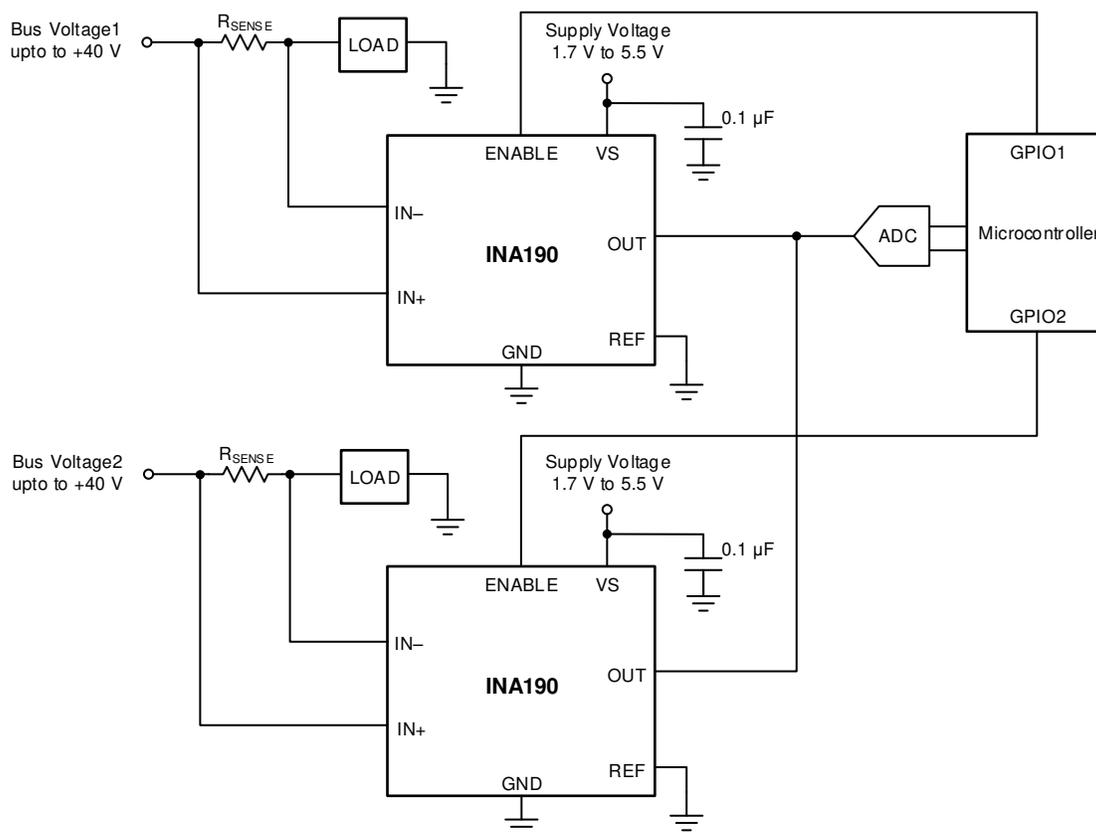
Figure 38. Multiplexing Multiple Devices With the ENABLE Pin
