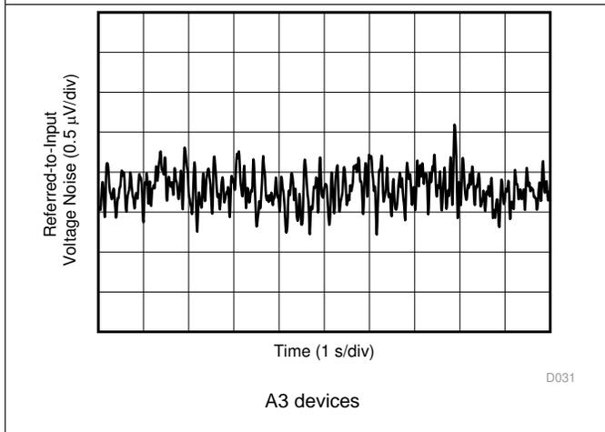
Figure 21. 0.1-Hz to 10-Hz Voltage Noise (Referred-To-Input)
