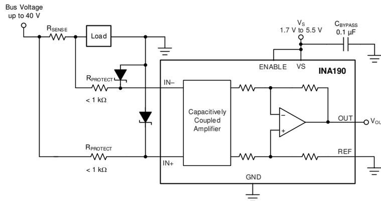
**Figure 42. Transient Protection Using Dual Zener Diodes**
