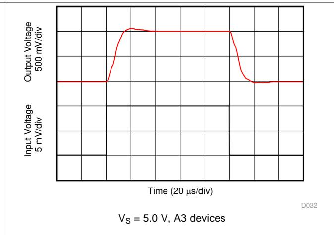
Figure 22. Step Response (10-mV<sub>PP</sub> Input Step)
