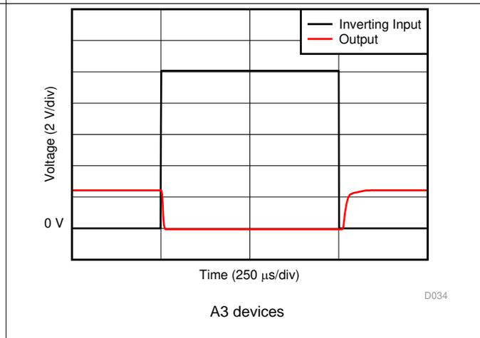
Figure 24. Inverting Differential Input Overload
