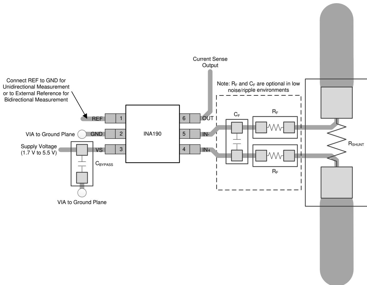
Figure 46. Recommended Layout for SC70 (DCK) Package
