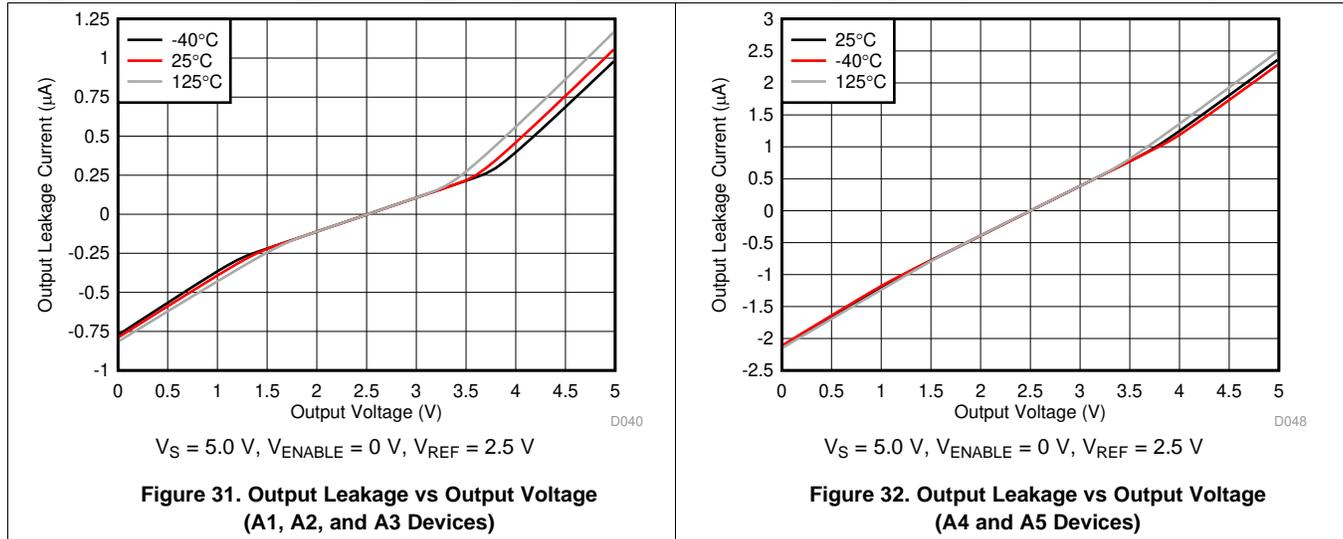
Figure 31. Output Leakage vs Output Voltage (A1, A2, and A3 Devices)
