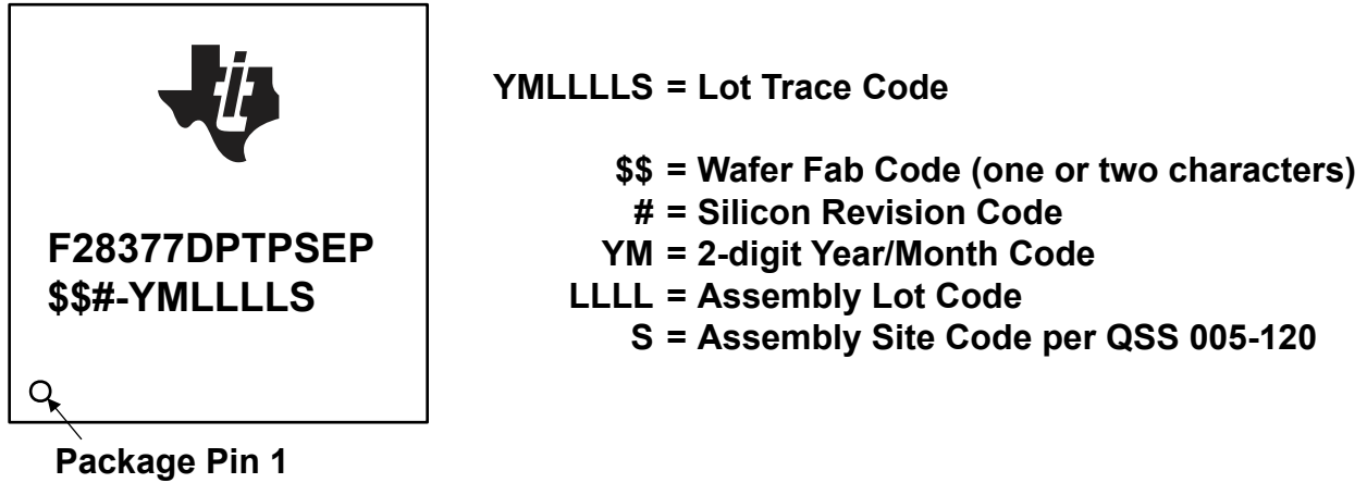
Figure 9-2. Example of Device Markings
