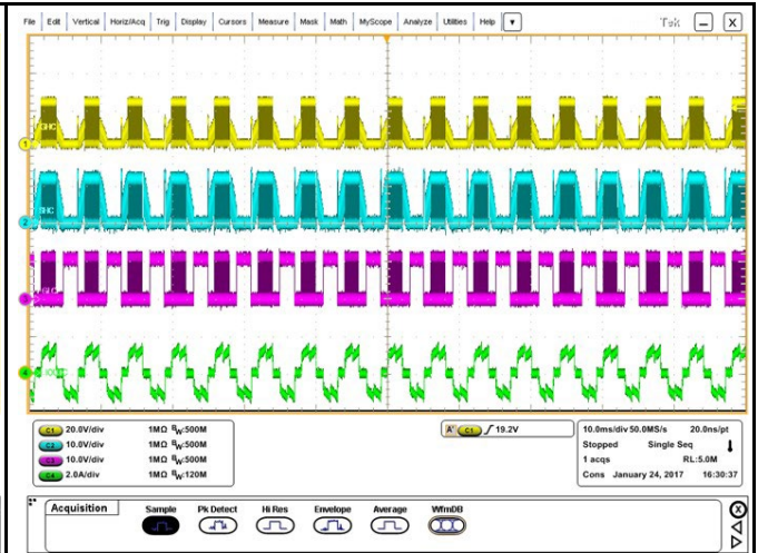
Figure 57. BLDC Motor Commutation 2000 RPM
