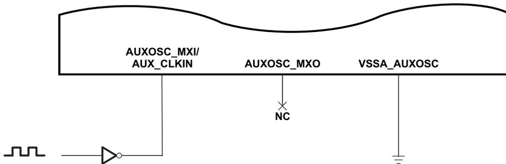
Figure 7-11. 1.8-V LVCMOS-Compatible Clock Input (AUX\_OSC)
