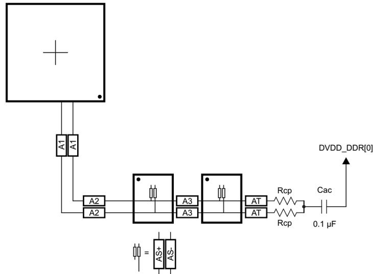
**Figure 8-68. CK Routing for Two Single-Side DDR3 Devices**
