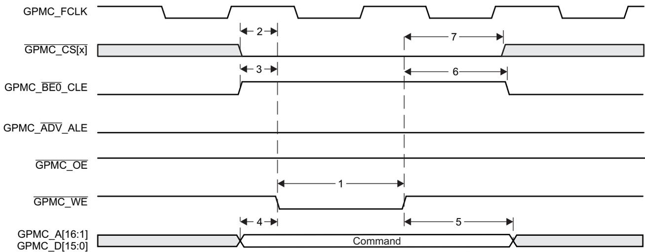
**Figure 8-33. GPMC/NAND Flash - Command Latch Cycle Timing**
