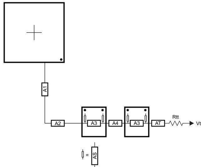
**Figure 8-65. ADDR\_CTRL Routing for Four Mirrored DDR3 Devices**
