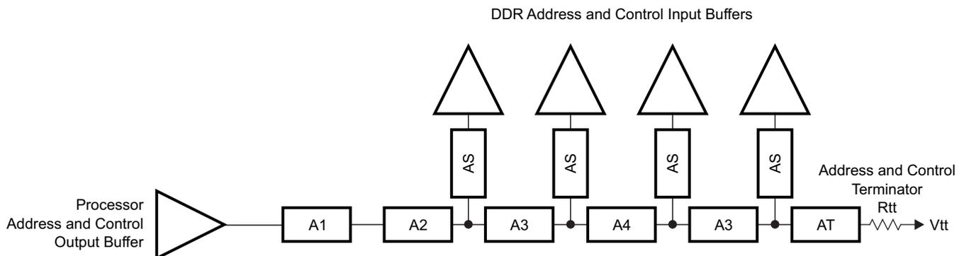
**Figure 8-61. ADDR\_CTRL Topology for Four x8 DDR3 Devices**
