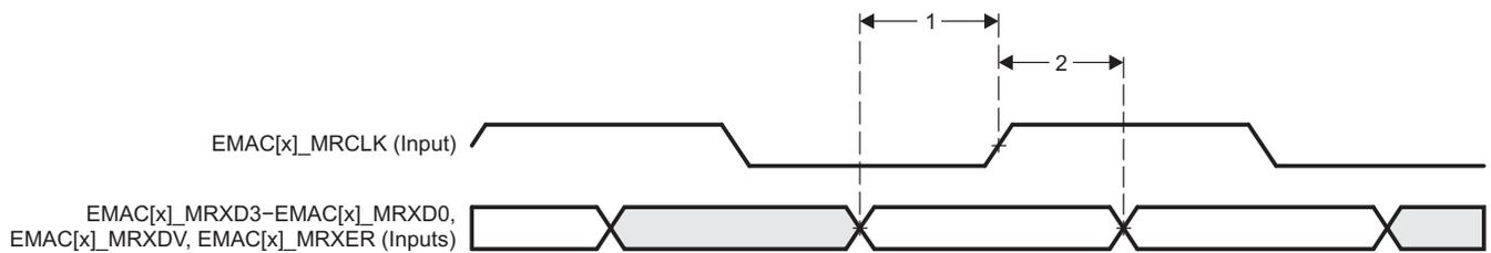
**Figure 8-11. EMAC Receive Interface Timing [G]MII Operation**
