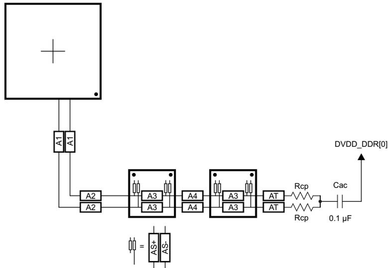
**Figure 8-64. CK Routing for Four Mirrored DDR3 Devices**
