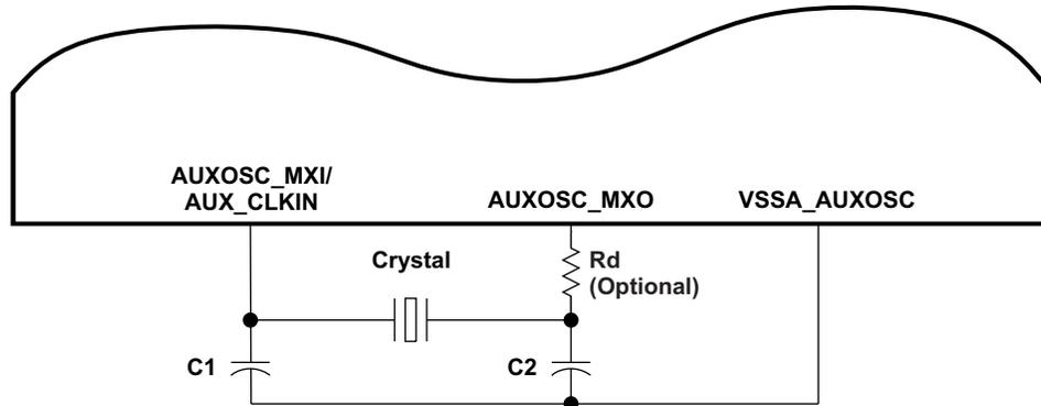
**Figure 7-9. Auxiliary Oscillator**
