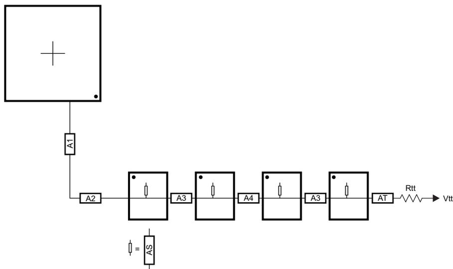
Figure 8-63. ADDR\_CTRL Routing for Four Single-Side DDR3 Devices
