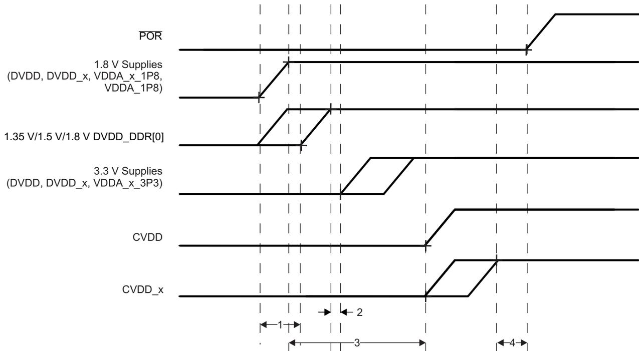
Both 1.8 V and DVDD\_DDR[x] supplies must be powered up and stable prior to starting the ramp of the 3.3 V supplies.
