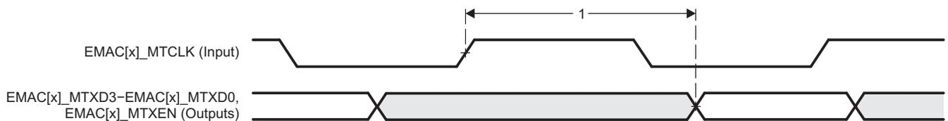
**Figure 8-12. EMAC Transmit Interface Timing [G]MII Operation**
