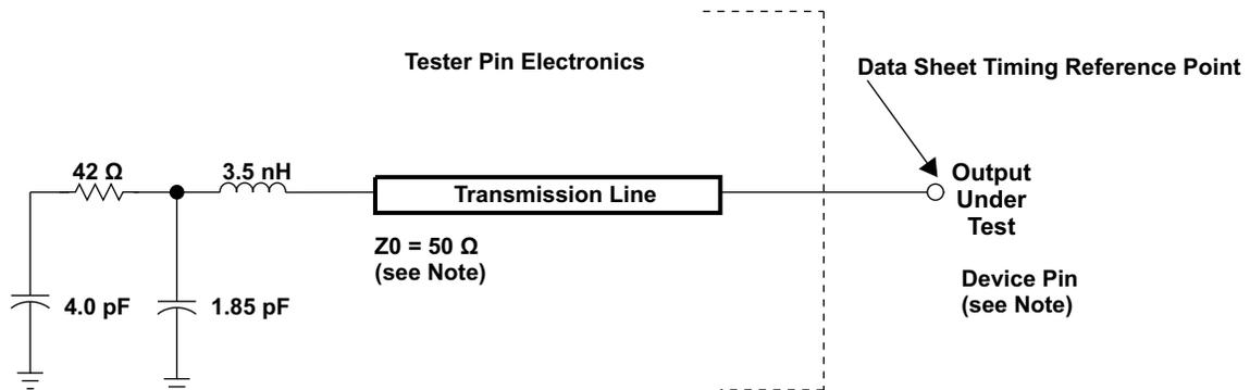
NOTE: The data sheet provides timing at the device pin. For output timing analysis, the tester pin electronics and its transmission line effects must be taken into account. A transmission line with a delay of 2 ns can be used to produce the desired transmission line effect. The transmission line is intended as a load only. It is not necessary to add or subtract the transmission line delay (2 ns) from the data sheet timings.
