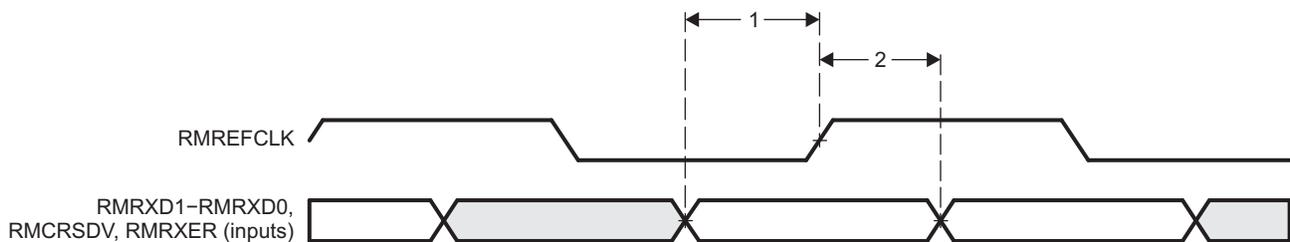
Figure 8-14. EMAC Receive Interface Timing RMII Operation
