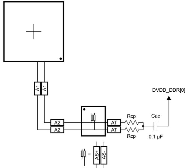
Figure 8-74. CK Routing for One DDR3 Device
