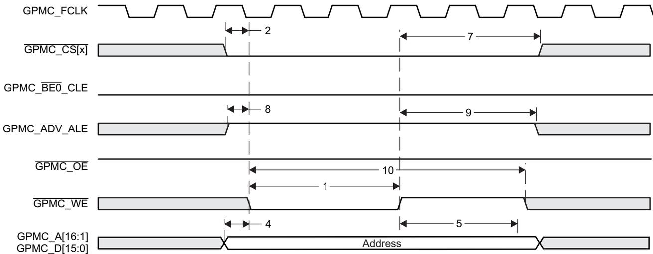
**Figure 8-34. GPMC/NAND Flash - Address Latch Cycle Timing**
