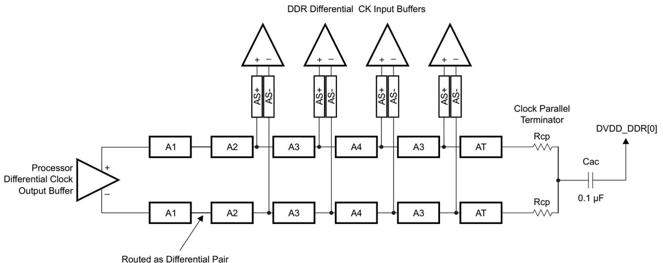
**Figure 8-60. CK Topology for Four x8 DDR3 Devices**
