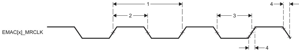
**Figure 8-9. EMAC[x]\_MRCLK Timing (EMAC Receive) - [G]MII Operation**
