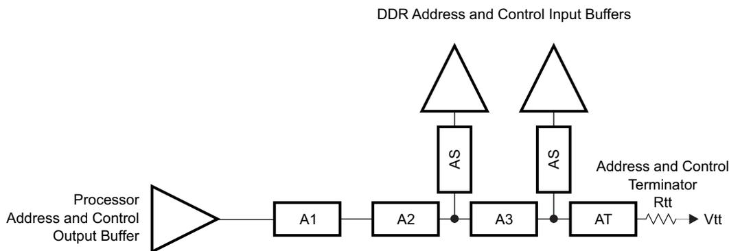
Figure 8-67. ADDR\_CTRL Topology for Two DDR3 Devices
