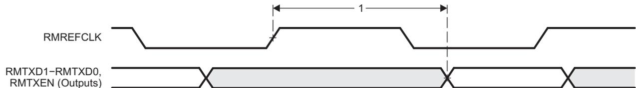
**Figure 8-15. EMAC Transmit Interface Timing RMII Operation**
