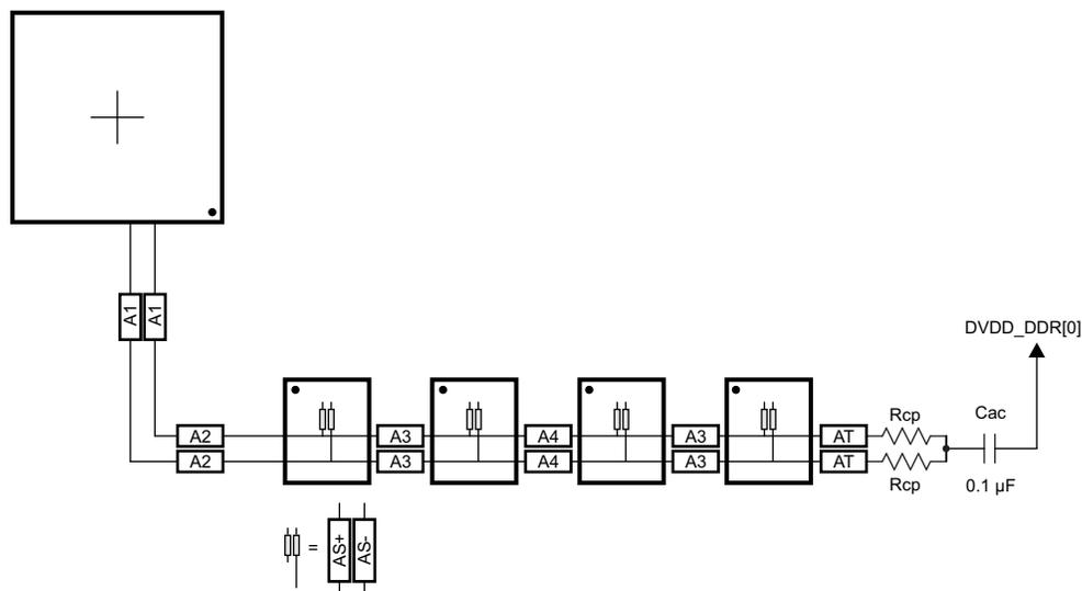
Figure 8-62. CK Routing for Four Single-Side DDR3 Devices
