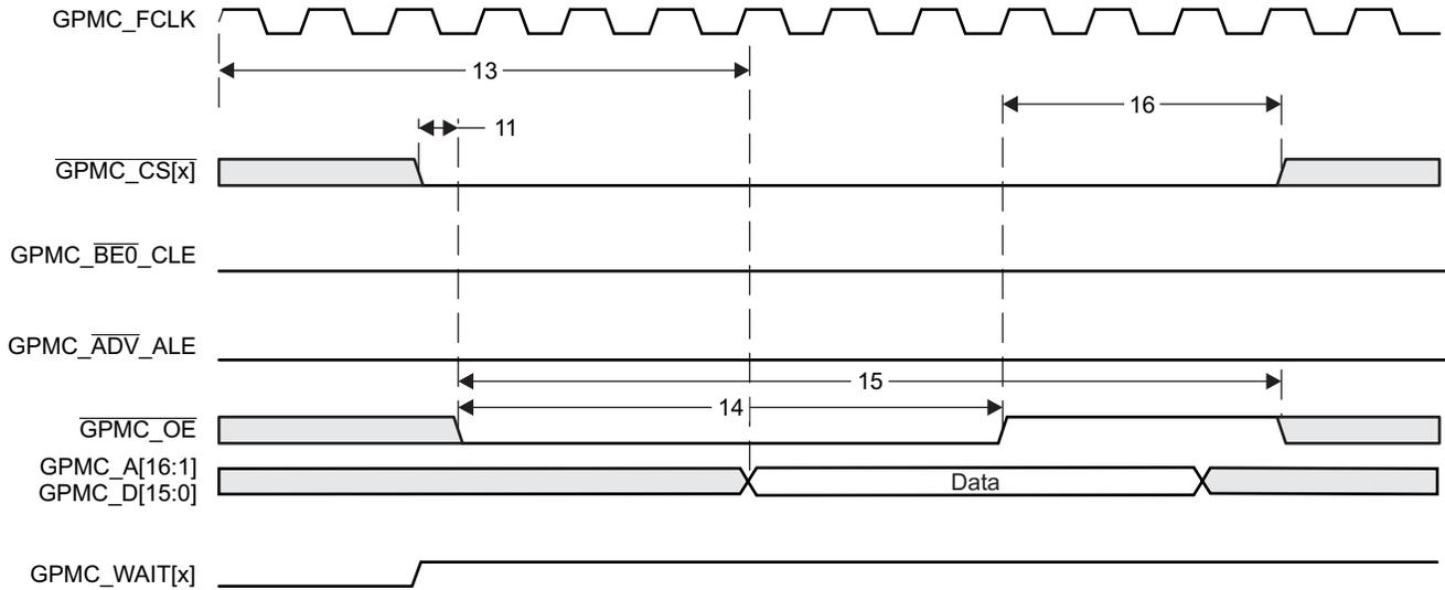
Figure 8-35. GPMC/NAND Flash - Data Read Cycle Timing
