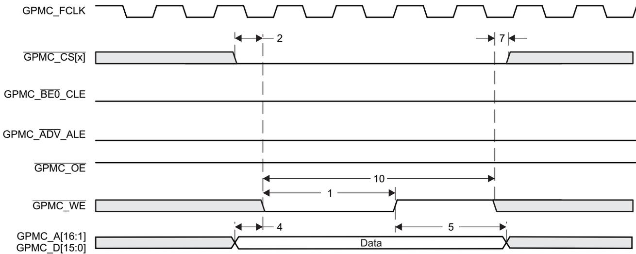
Figure 8-36. GPMC/NAND Flash - Data Write Cycle Timing
