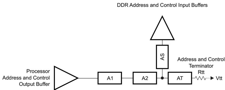
Figure 8-73. ADDR\_CTRL Topology for One DDR3 Device
