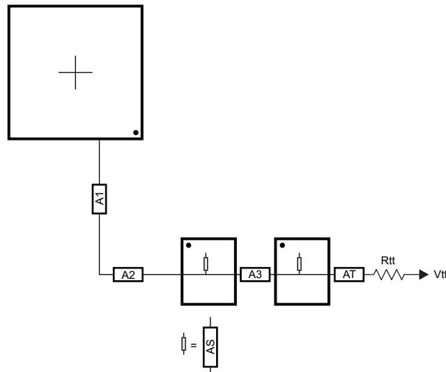
**Figure 8-69. ADDR\_CTRL Routing for Two Single-Side DDR3 Devices**
