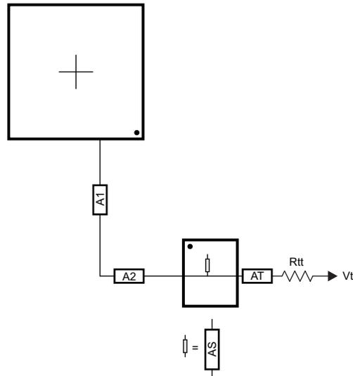
Figure 8-75. ADDR\_CTRL Routing for One DDR3 Device
