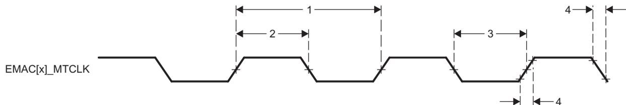
**Figure 8-10. EMAC[x]\_MTCLK Timing (EMAC Transmit) - [G]MII Operation**
