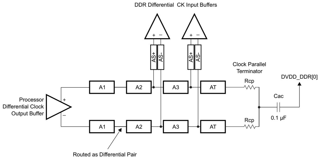
Figure 8-66. CK Topology for Two DDR3 Devices
