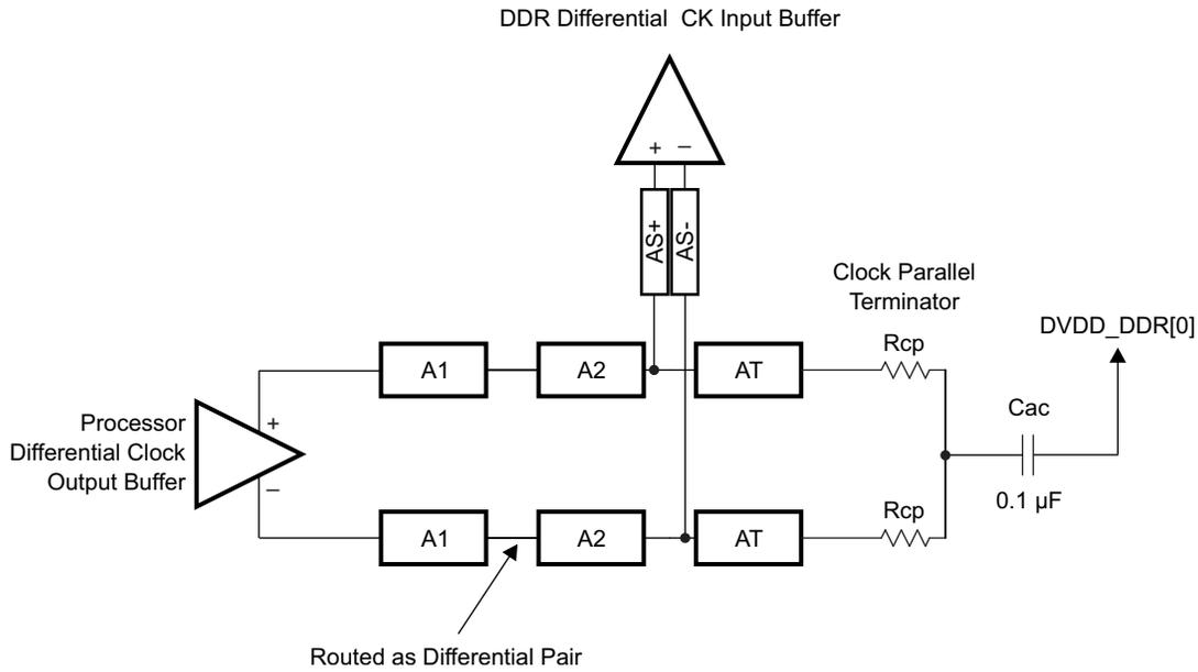
Figure 8-72. CK Topology for One DDR3 Device
