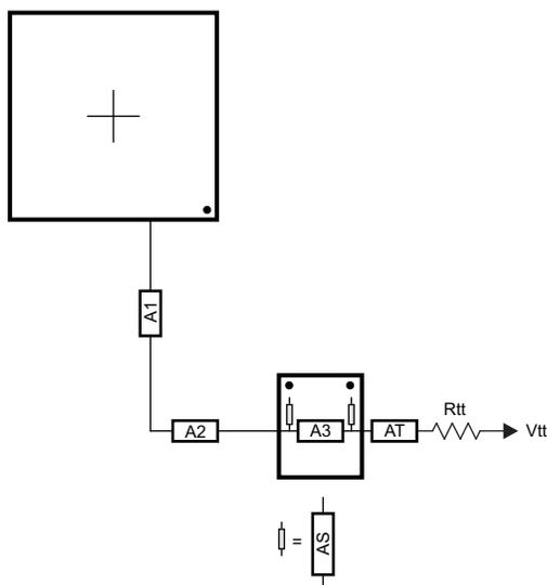
Figure 8-71. ADDR\_CTRL Routing for Two Mirrored DDR3 Devices
