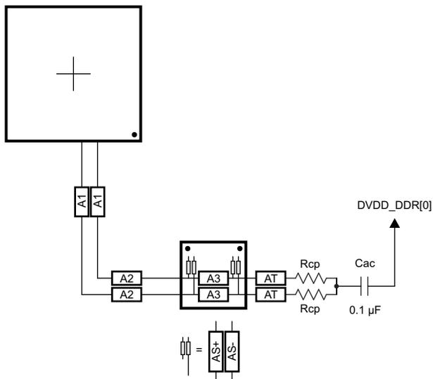
Figure 8-70. CK Routing for Two Mirrored DDR3 Devices
