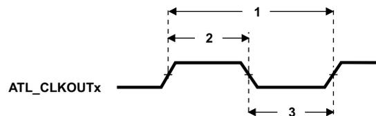
**Figure 8-4. ATL\_CLKOUTx Timing**
