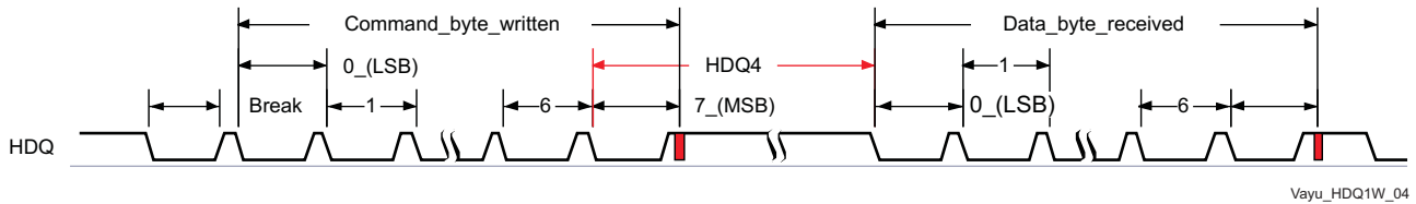
Figure 5-45. HDQ Communication Timing
