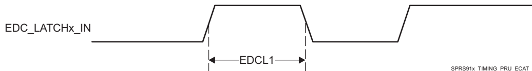
Figure 5-120. PRU-ICSS ECAT LATCHx_IN Timing
