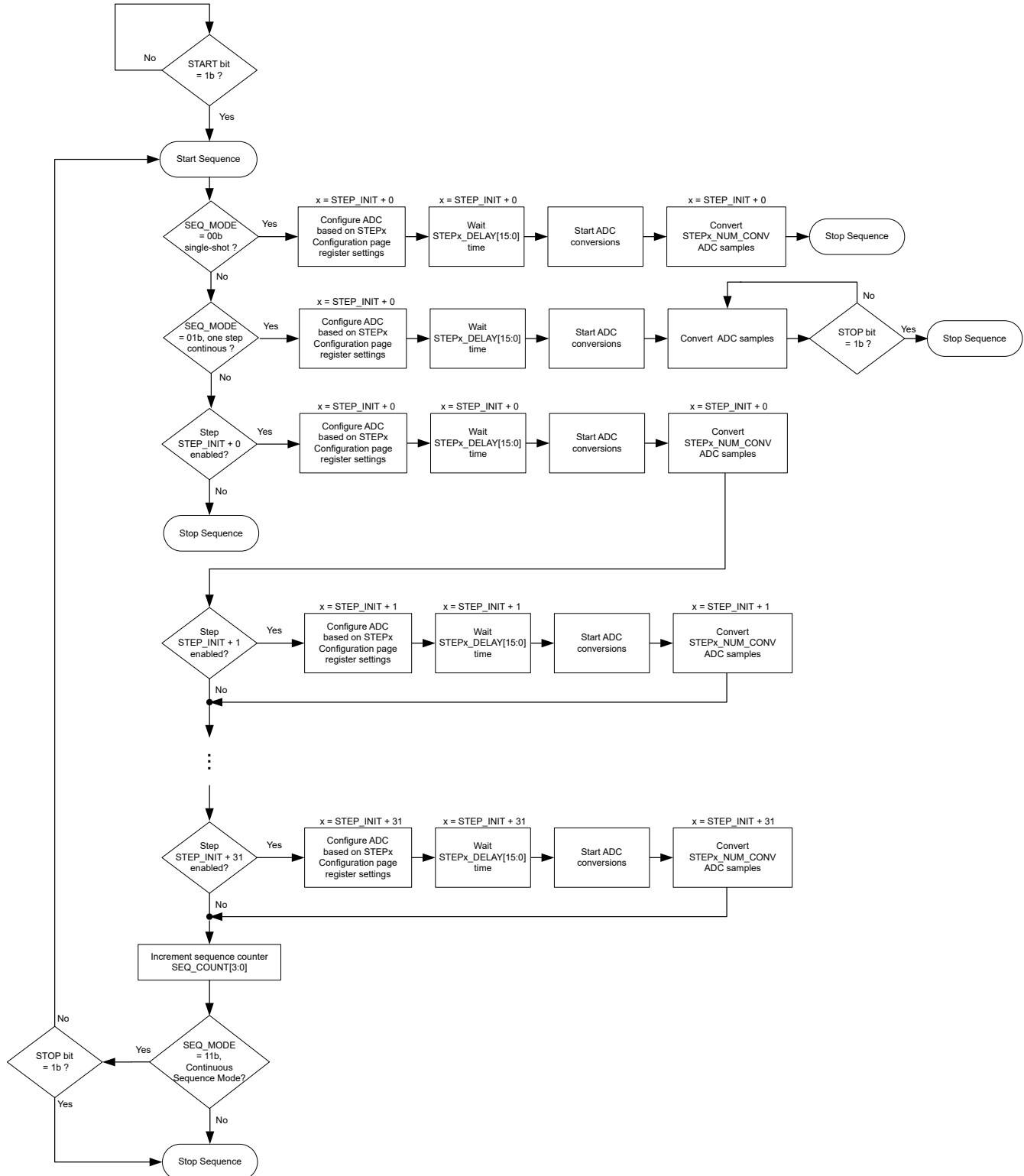
Figure 7-21. Sequencer Flow Chart
