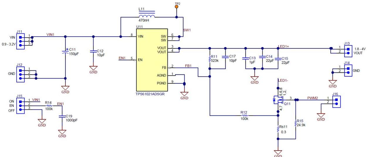
**Figure 2.2 Schematic of the PMP15037 (PWM Dimming)**
