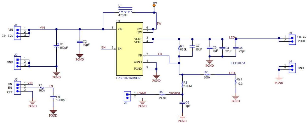
**Figure 2.1 Schematic of the PMP15037 (Analog Dimming)**
