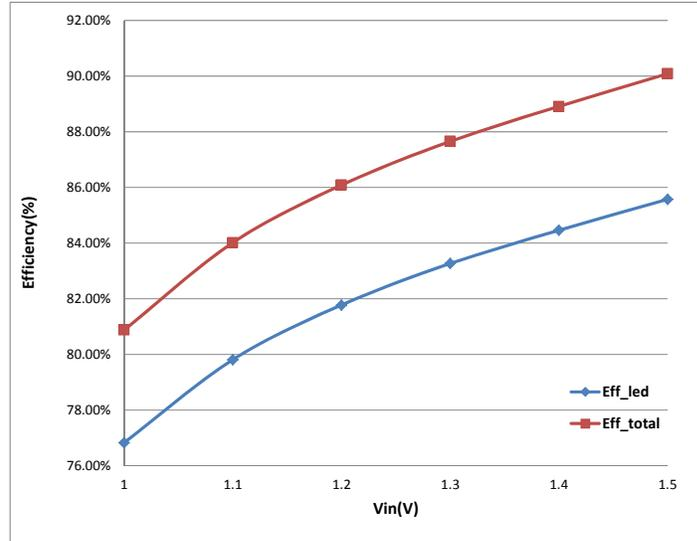
**Figure 4. Conversion Efficiency under Analog Dimming (Io=0.5A)**
