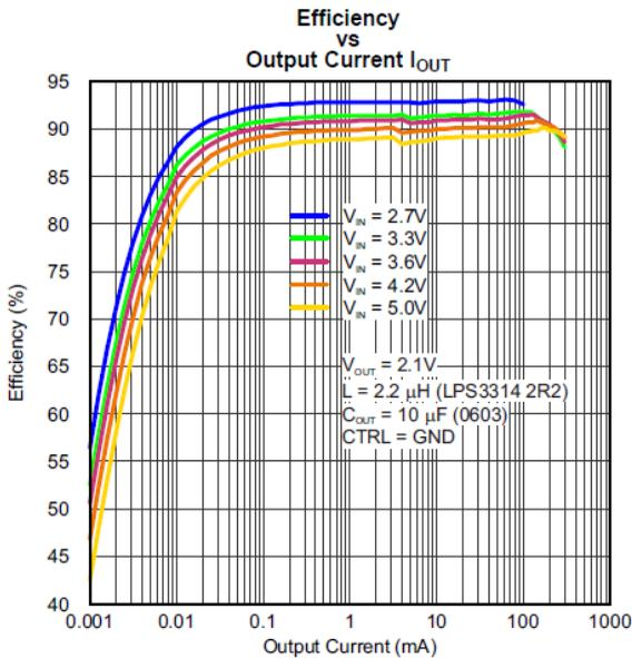
Figure 8. Efficiency V<sub>OUT</sub> = 2.1V
