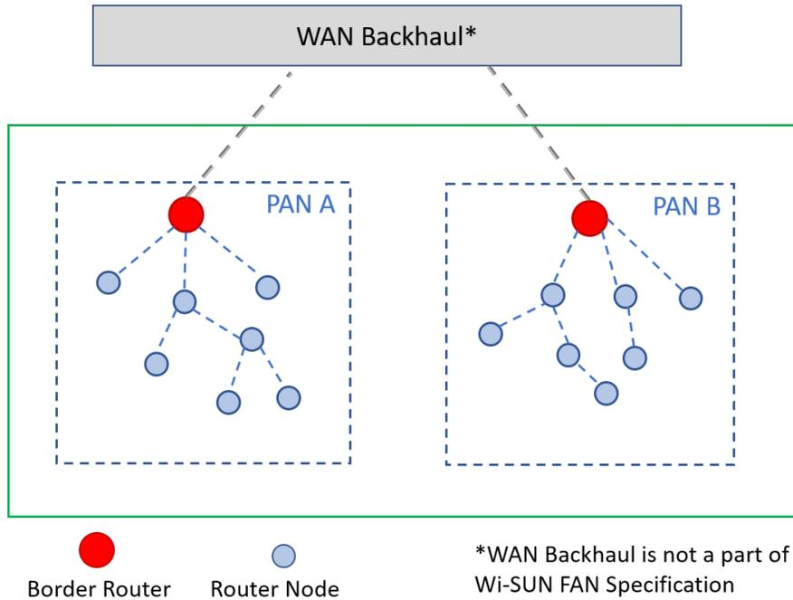
**Figure 2. Wi-SUN® Network Topology Consisting of Two PANs**
