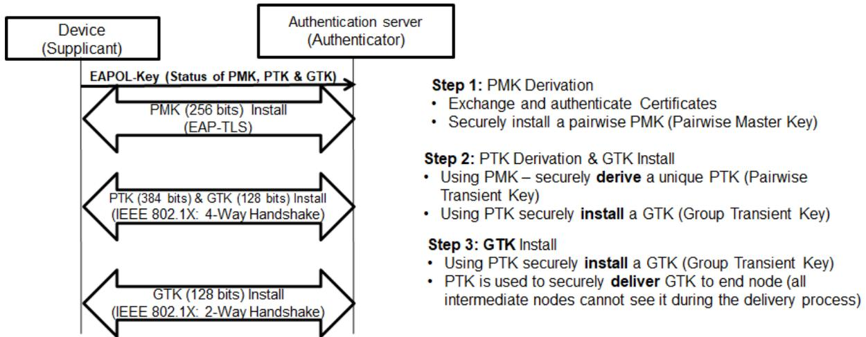
Figure 3. Security Key Exchange Mechanism in Wi-SUN®
