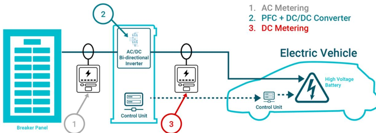
Figure 1. Metering and current sensing inside AC/DC chargers
