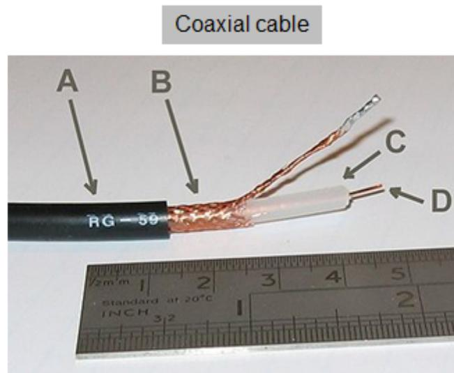
**Figure 5. Coaxial Cable Close-up: the Outer Plastic Sheath (a); Woven Copper Shield (Ground) (b); Inner Dielectric Insulator (c); and Copper Core ( $V_{OUT}$ ) (d)**
