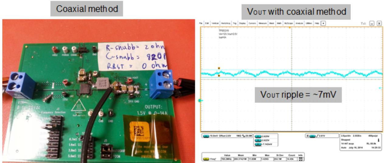
**Figure 4. Output-voltage Ripple Probe Using Coaxial Method**
