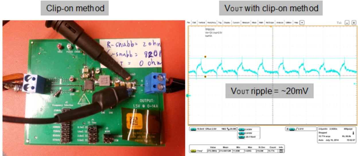
**Figure 2. Output Voltage Ripple Probe with a Clip-on Probe and Ground Wire Fully Extended, Picking up Noise from the Nearby Switch Node**
