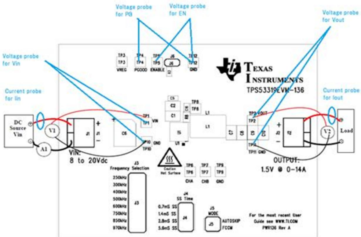
Figure 1. Output-voltage Ripple Probe Setup
