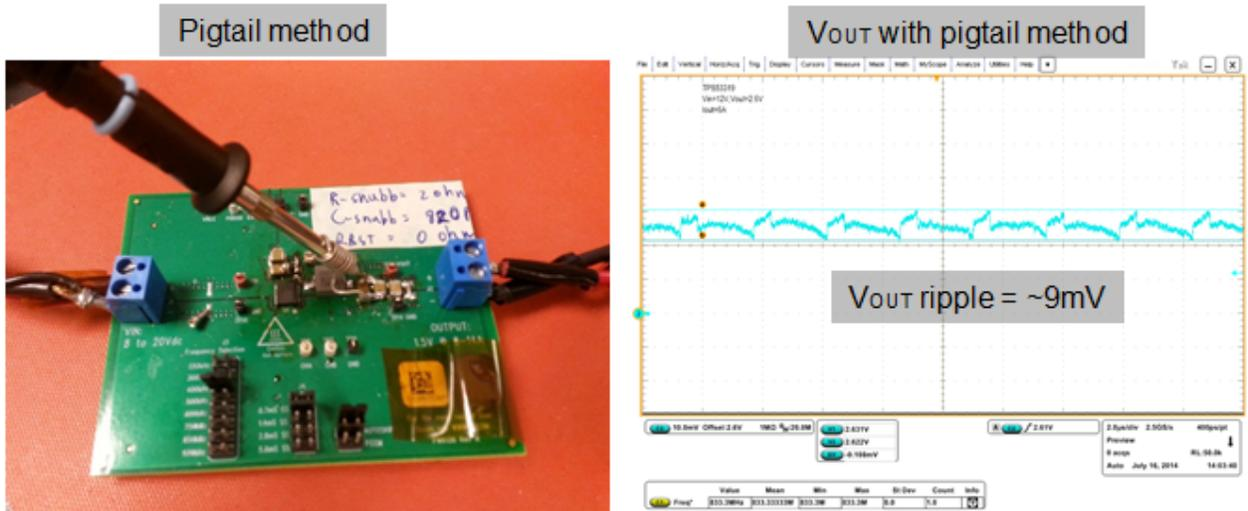
**Figure 3. Output-voltage Ripple Probe Using the Pigtail Method; the Probe Ground Is in Contact with the Pigtail, Which Is Connected to the Board Ground**
