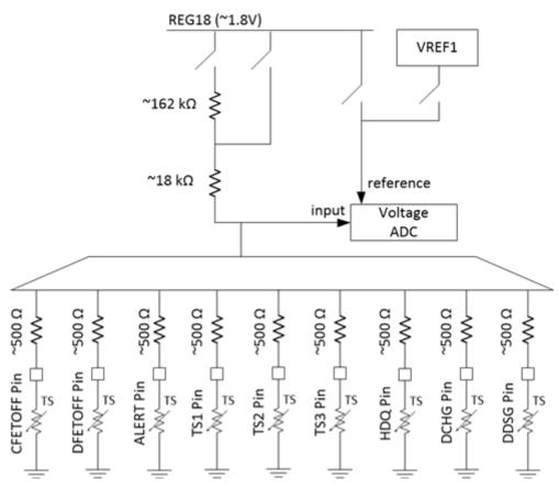
Figure 1. Temperature Measurement Using External Thermistors
