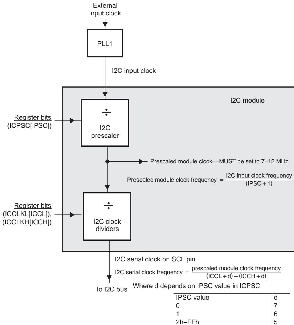
The prescaler (ICPSC [IPSC]) must only be initialized while the I2C module is in the reset state (ICMDR [IRS] = 0). The prescaled frequency only takes effect when ICMDR [IRS] is changed to 1. Changing the ICPSC [IPSC] value while ICMDR [IRS] = 1 has no effect. Likewise, you must configure the I2C clock dividers (ICCLKH [ICCH] and ICCLKL [ICCL]) while the I2C module is still in reset (ICMDR [IRS] = 0).
