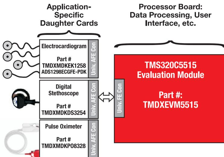
▲ Figure 1: TMS320C5515 Medical Development Kits system block diagram
