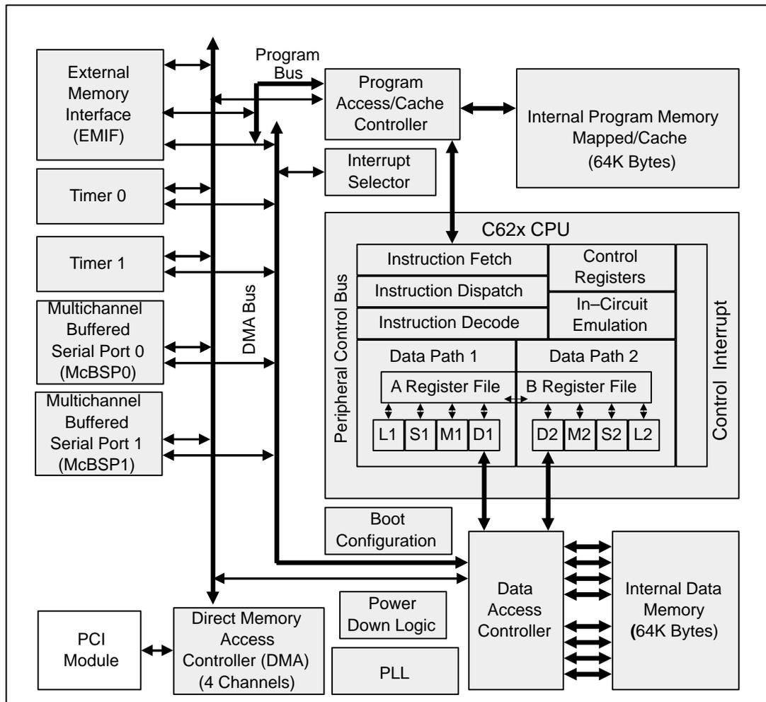
Figure 2. TMS320C6205 DSP Block Diagram
