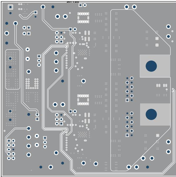
**Figure 8-7. TPS546B24AEVM-2PH Internal Layer 2 (Top View)**
