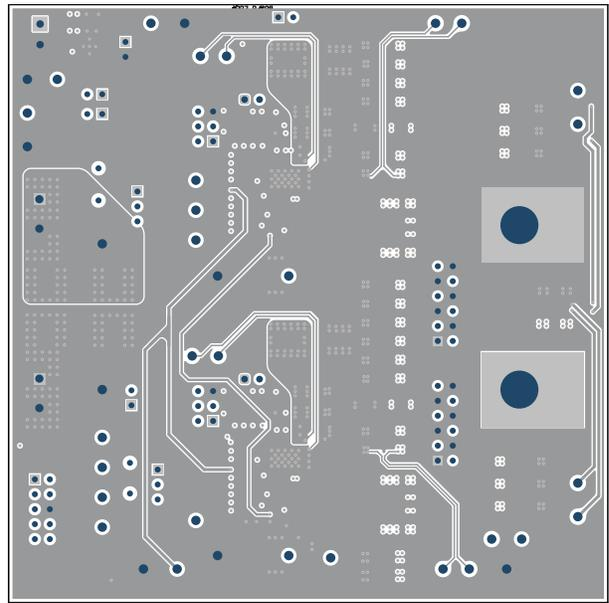
Figure 8-10. TPS546B24AEVM-2PH Internal Layer 5 (Top View)
