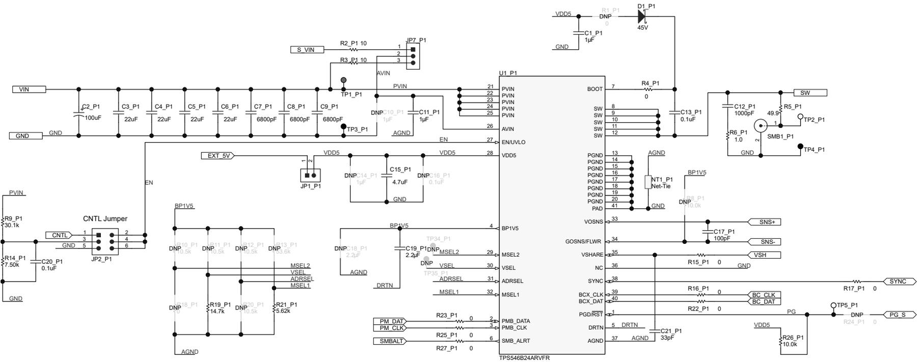
Figure 3-2. TPS546B24AEVM-2PH Schematic Page 2 (U1\_P1 Loop Controller)
