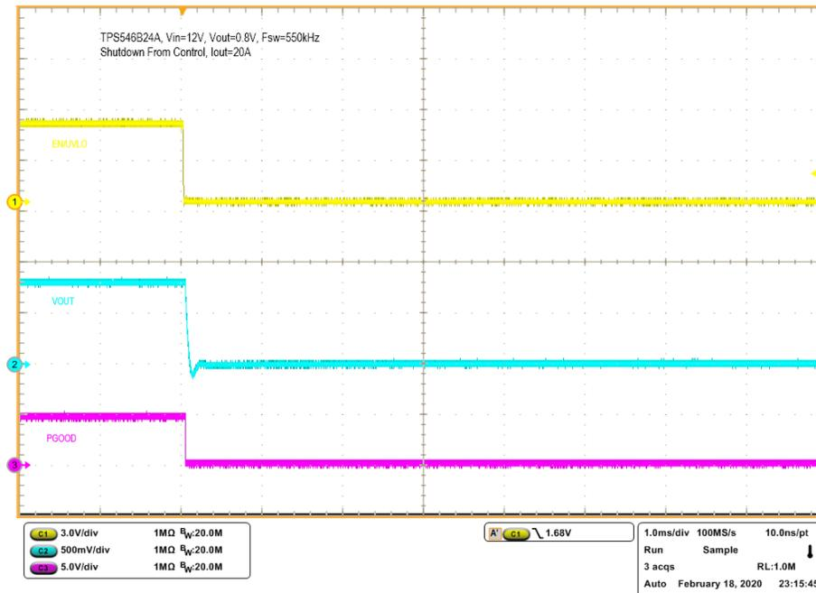
Figure 7-14. Shutdown From Control, 20-A CC Load
