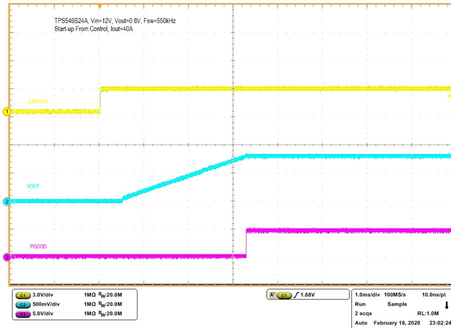
Figure 7-12. Start-Up From Control, 40-A CC Load
