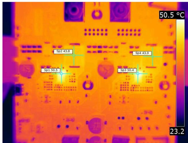
$V_{IN} = 12\text{ V}$ ,  $I_{OUT} = 40\text{ A}$
