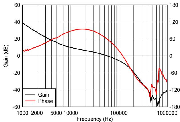
Figure 7-6. Bode Plot at 0.8-V Output at 12 V<sub>IN</sub>, 20-A Load
