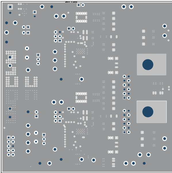
Figure 8-11. TPS546B24AEVM-2PH Internal Layer 6 (Top View)
