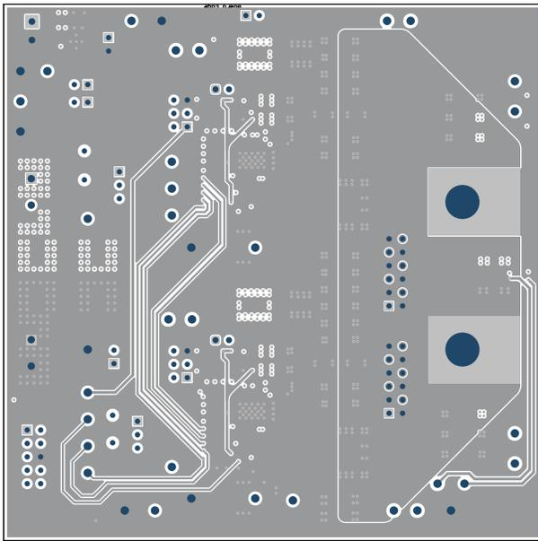
Figure 8-9. TPS546B24AEVM-2PH Internal Layer 4 (Top View)
