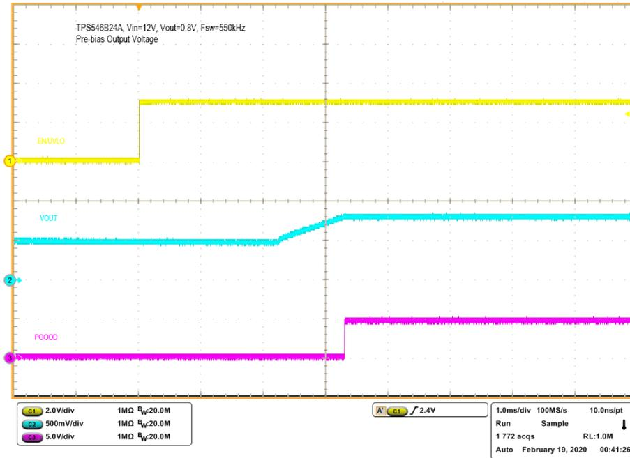
Figure 7-15. Start-Up From Control With Pre-Biased Output
