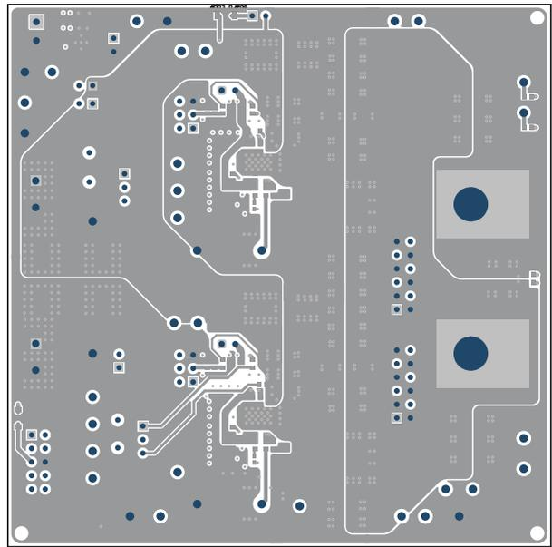
Figure 8-12. TPS546B24AEVM-2PH Internal Bottom Layer (Top View)
