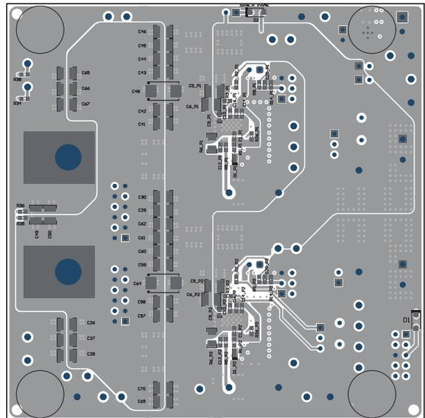
Figure 8-4. TPS546B24AEVM-2PH Bottom Side Component View (Bottom View)
