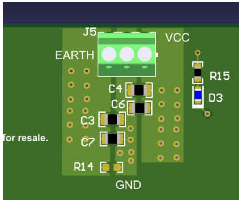
**Figure 4-1. Power Connection Block View: J5**
