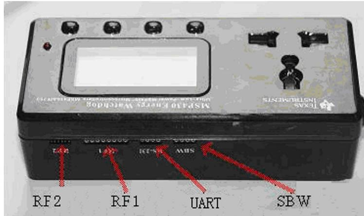
**Figure 4. Interface Ports on the MSP430 Energy Watchdog Tool**
