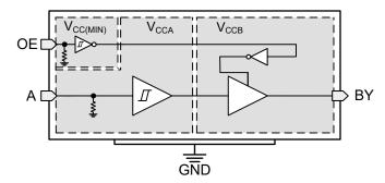
Figure 1-1. Functional Block Diagram
