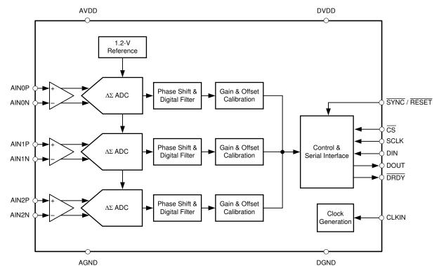
Figure 1-1. Functional Block Diagram
