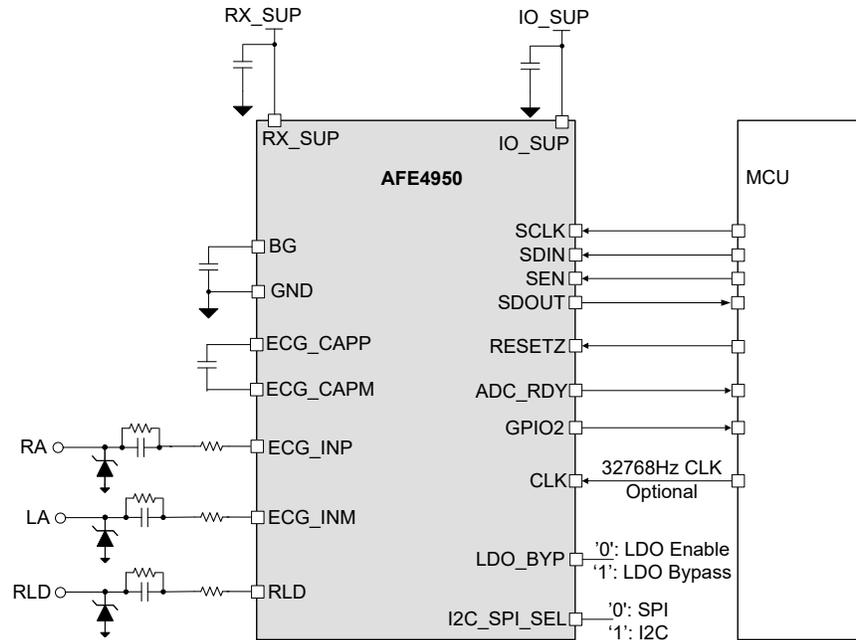
**Figure 3. Reference Schematic of an ECG Acquisition System Using AFE4950**
