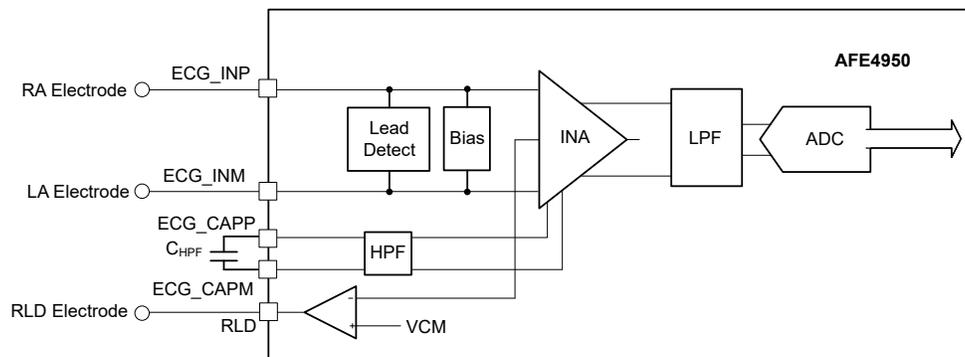
**Figure 4. AFE4950 Signal Chain for ECG Signal Acquisition**
