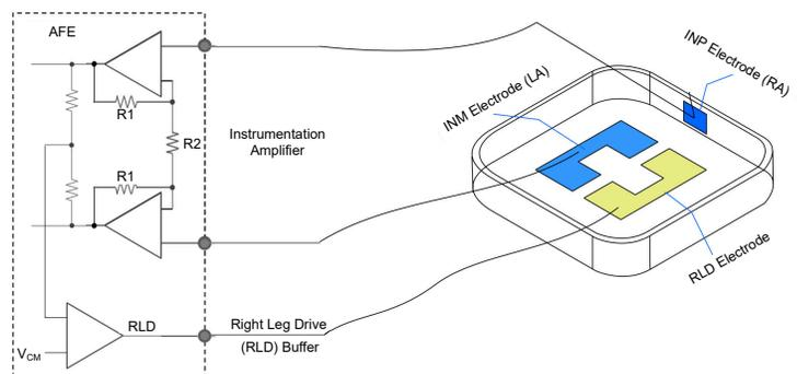
Figure 2. Interface of the AFE to the Three ECG Electrodes
