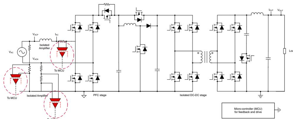
**Figure 1. Implementation of a Server Power Supply With PFC and DC-DC Stages**
