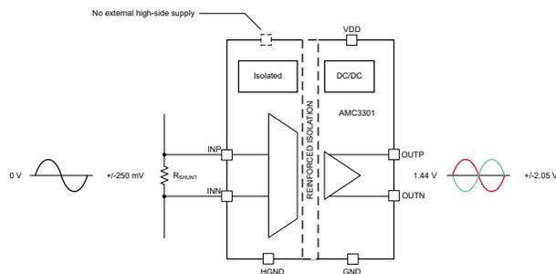
**Figure 2. AMC3301 Block Diagram**
