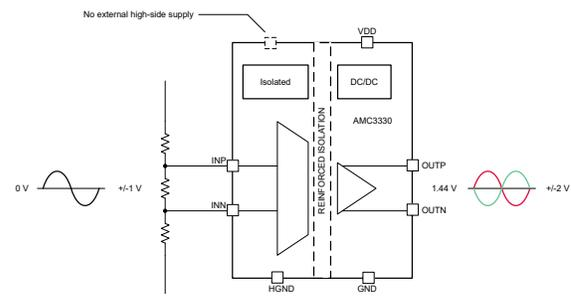
**Figure 3. AMC3330 Block Diagram**
