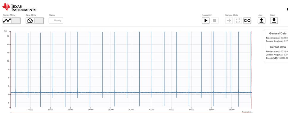
☒ 22. Collector Current Consumption for a Beacon Interval of 1.23 s
