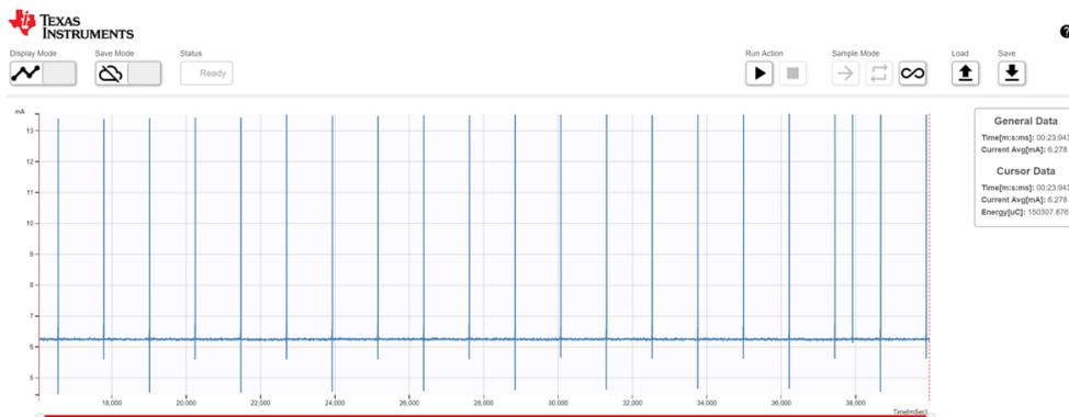
図 24. Collector Current Consumption for +10-dBm Transmit Power
