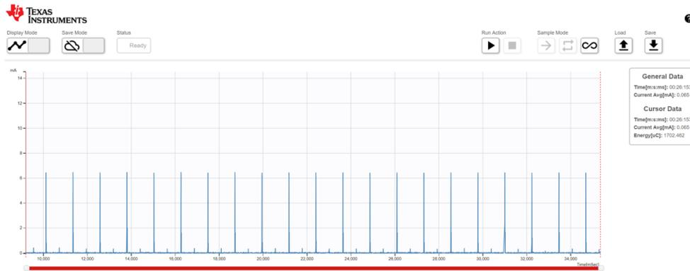
☒ 19. Sensor Current Consumption for a Beacon Interval of 1.23 s
