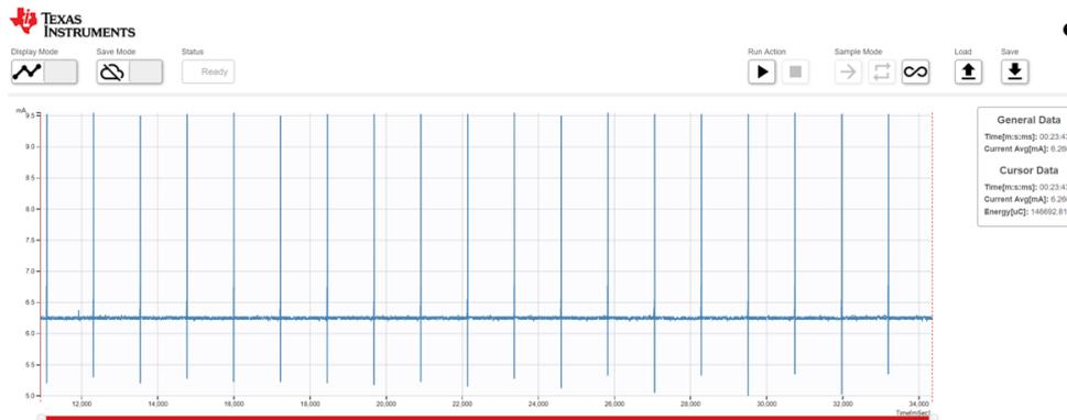
☒ 25. Collector Current Consumption for +6-dBm Transmit Power
