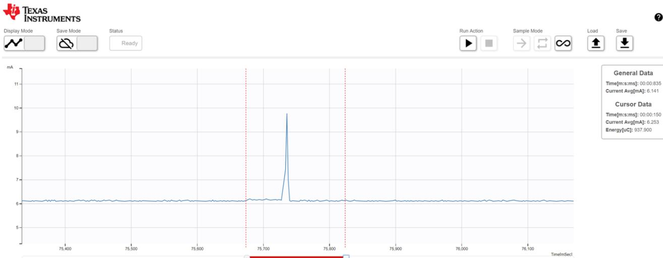
☒ 36. Collector Current Consumption for Receiving 300-Byte Data
