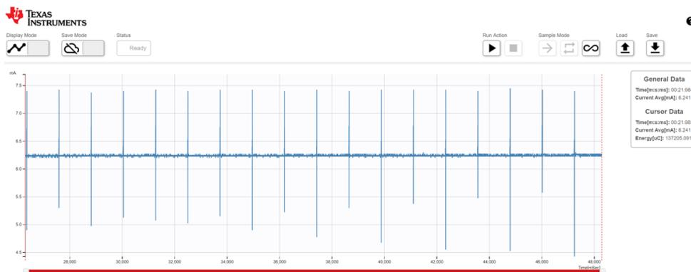
☒ 26. Collector Current Consumption for 0-dBm Transmit Power
