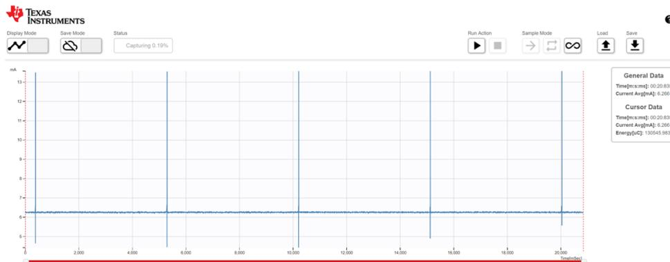
☒ 21. Collector Current Consumption for a Beacon Interval of 4.92 s
