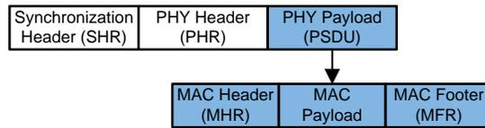
図 3. Schematic View of PDU
