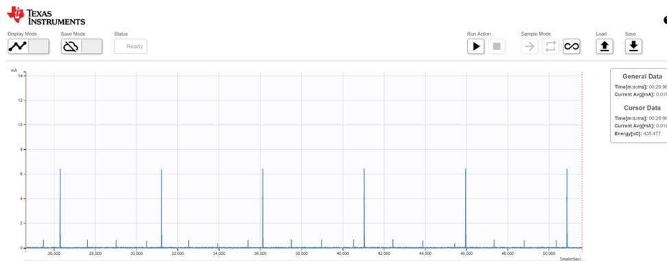
**図 18. Sensor Current Consumption for a Beacon Interval of 4.92 s**
