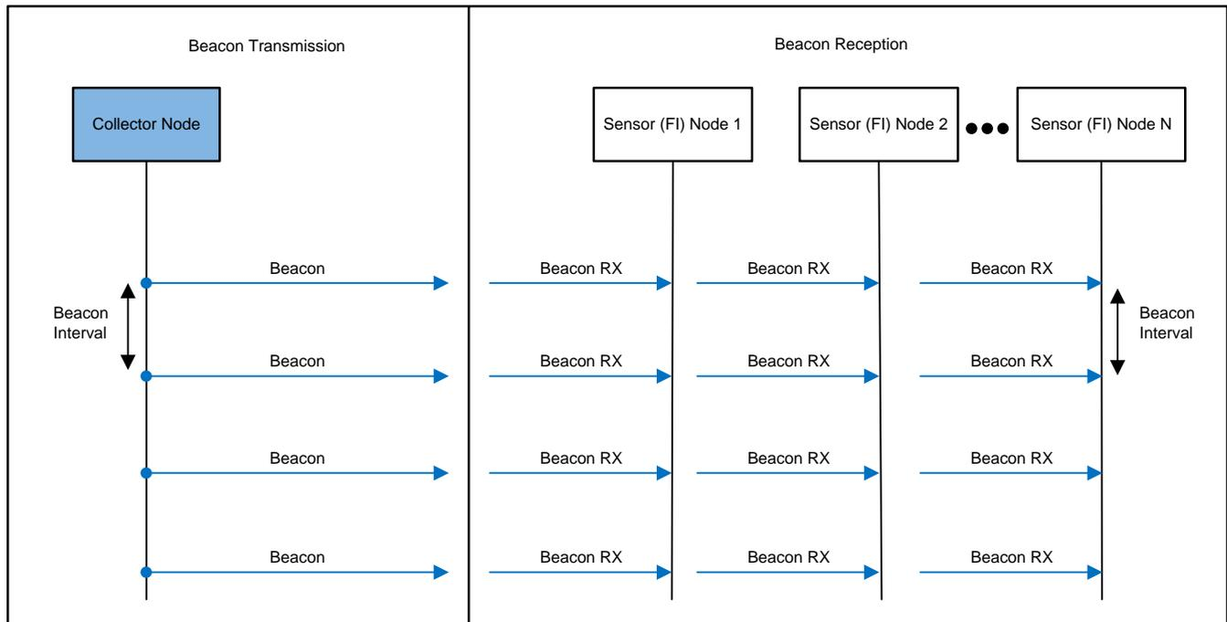
All Sensor (FI) nodes connected to the PAN will track the beacon and enable RX just before the start of the Beacon.
