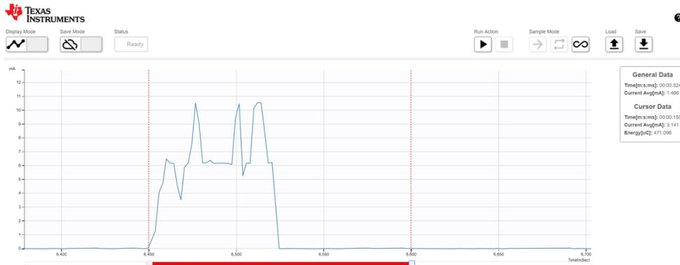
☒ 27. Sensor Current Consumption for Reception of 1-Byte Data
