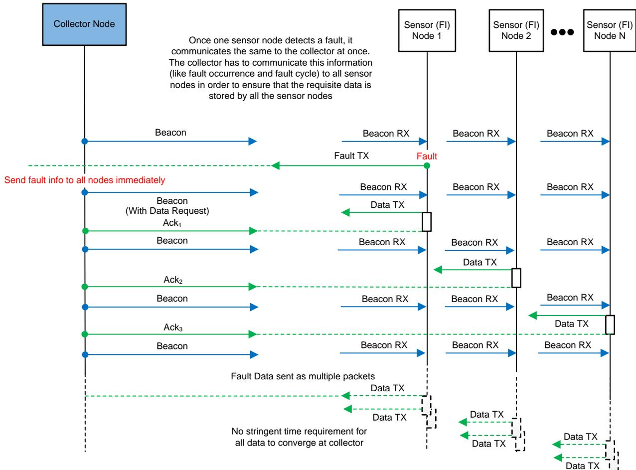
図 16. Fault Detection and Fault Information Broadcast
