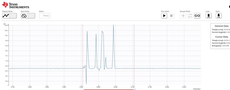
Figure 30. Collector Current Consumption for Transmission of 1-Byte Data
