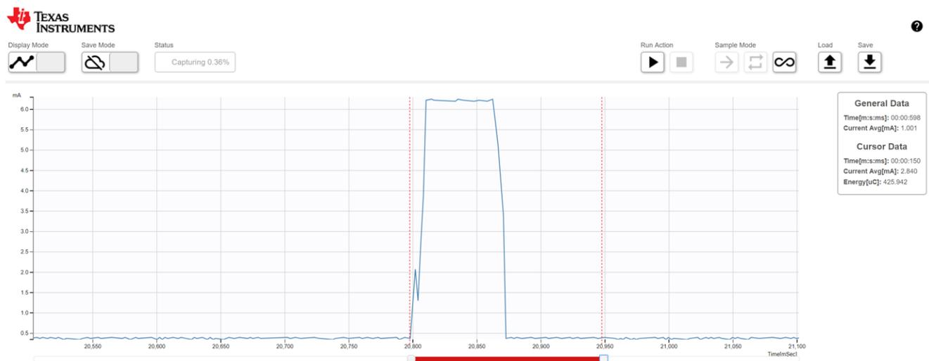
☒ 34. Sensor Current Consumption for Transmitting 300-Byte Data
