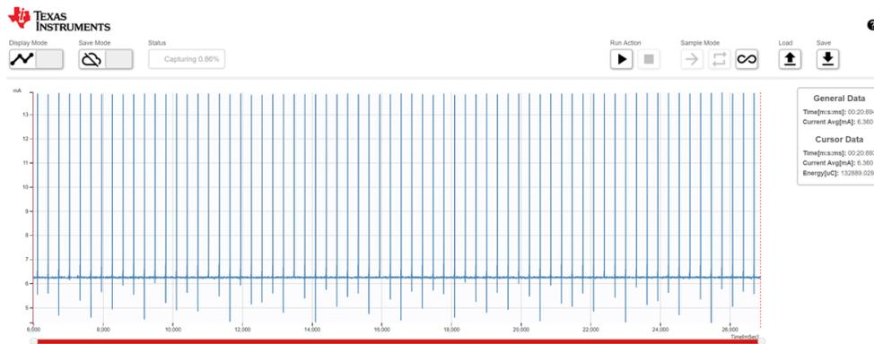
図 23. Collector Current Consumption for a Beacon Interval of 0.31 s
