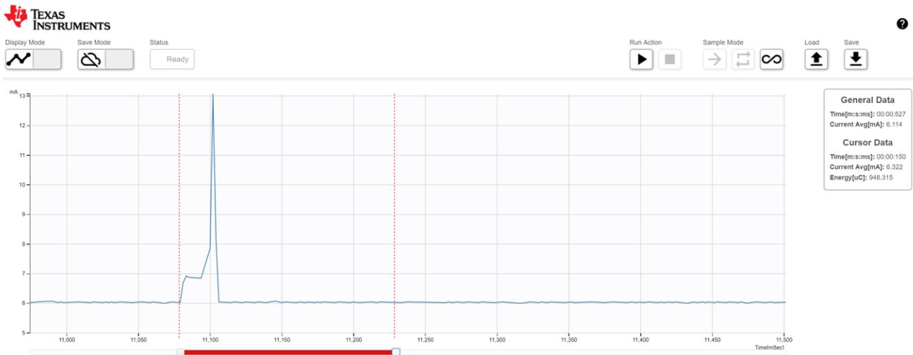
☒ 35. Collector Current Consumption for Receiving 70-Byte Data
