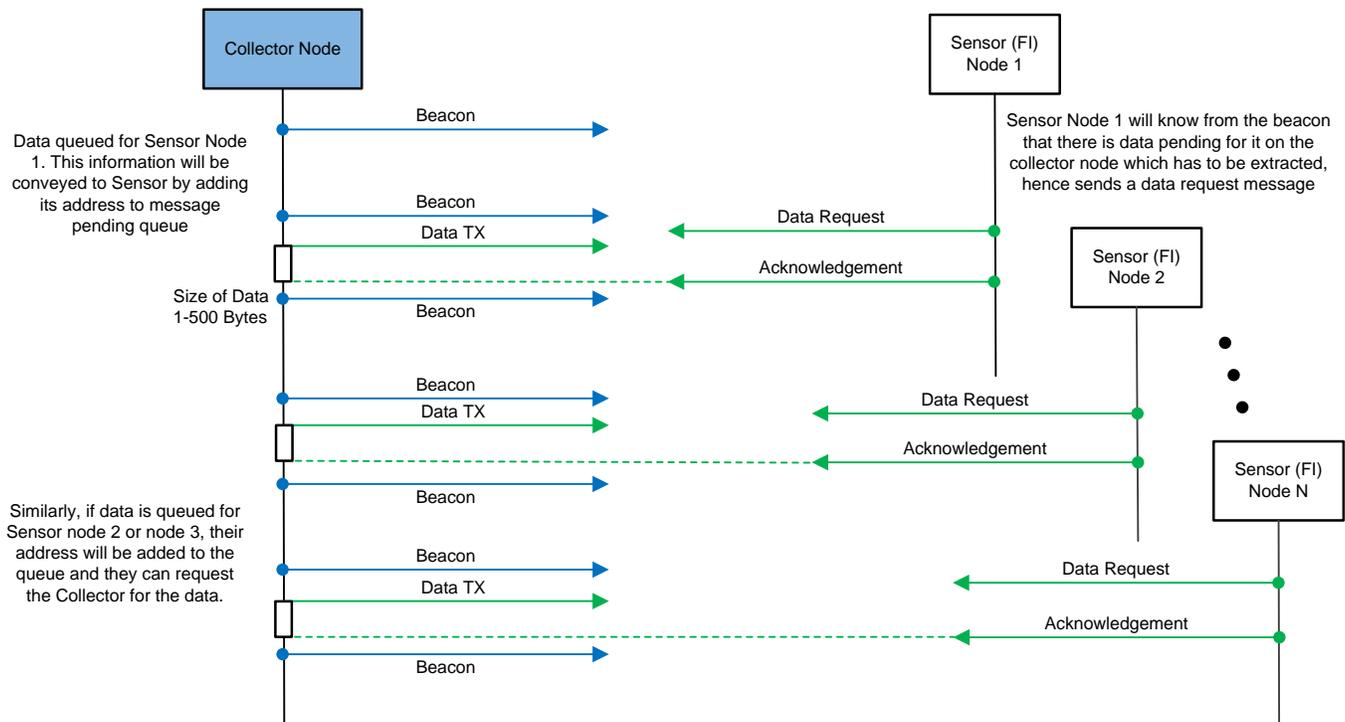
図 15. Data Exchange Between Sensor and Collector
