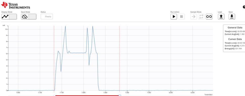
☒ 28. Sensor current consumption for reception of 150-Byte Data
