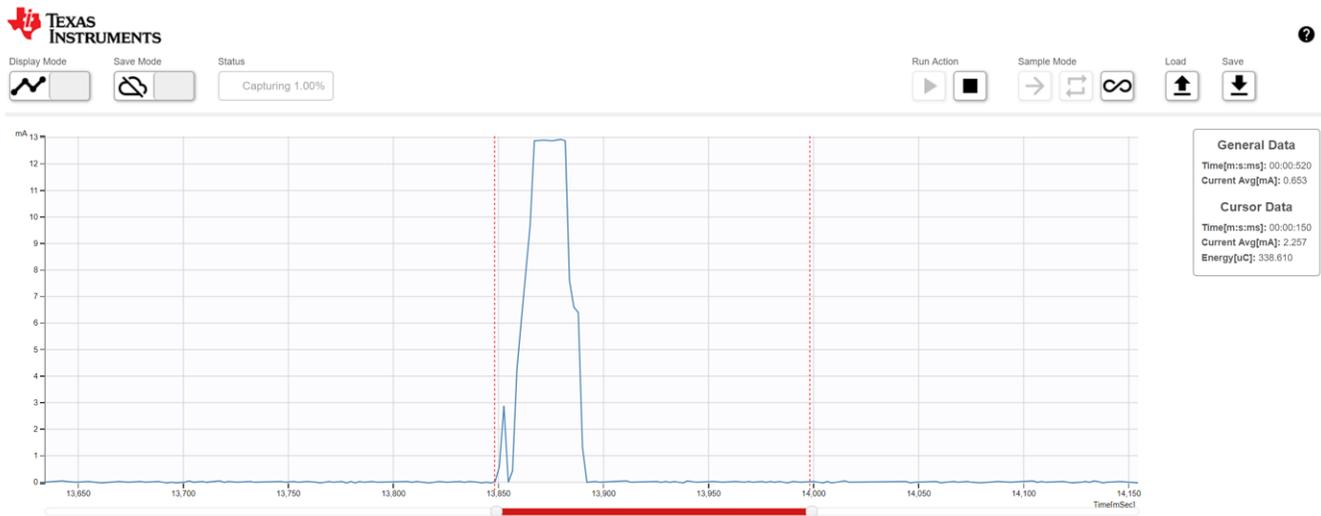
☒ 33. Sensor Current Consumption for Transmitting 70-Byte Data
