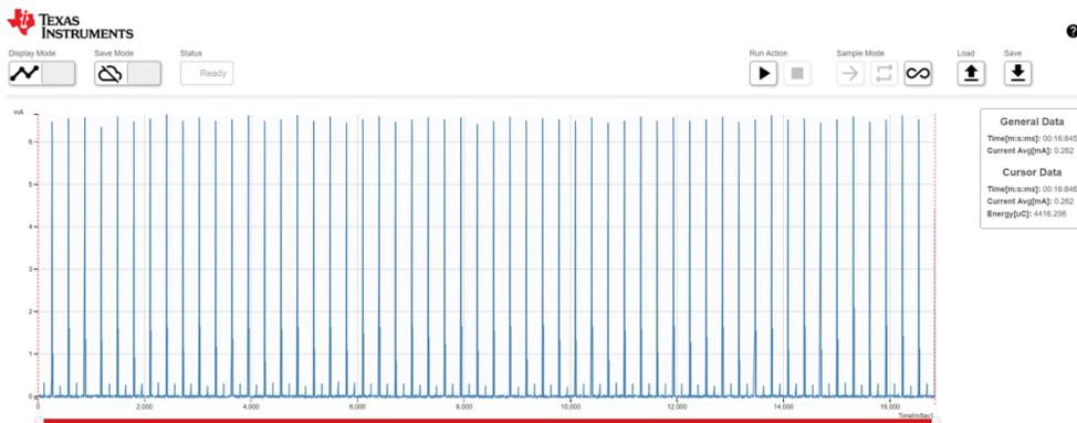
☒ 20. Sensor Current Consumption for a Beacon Interval of 0.31 s
