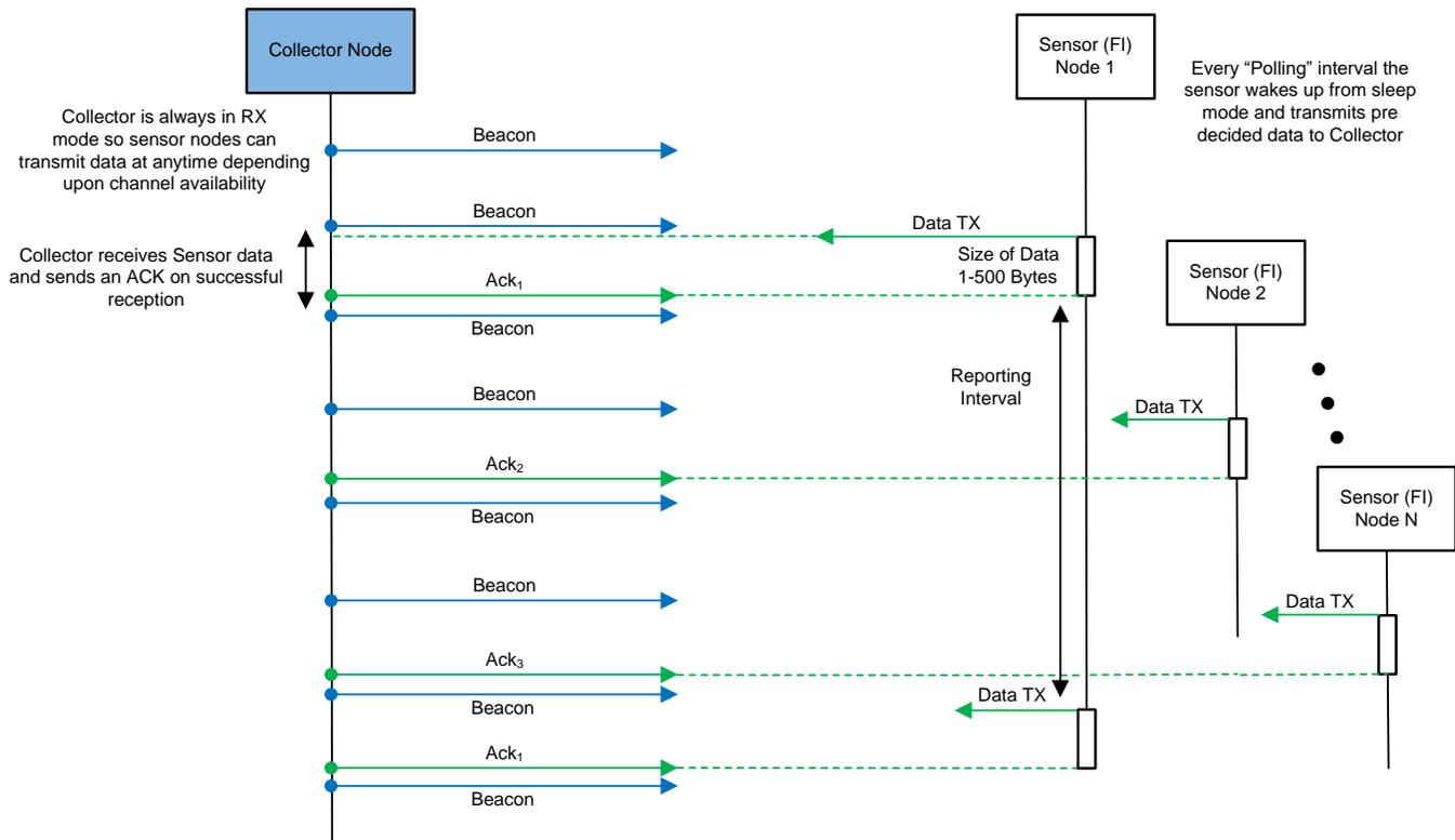
図 14. Status Report From Sensor (FPI) to Collector
