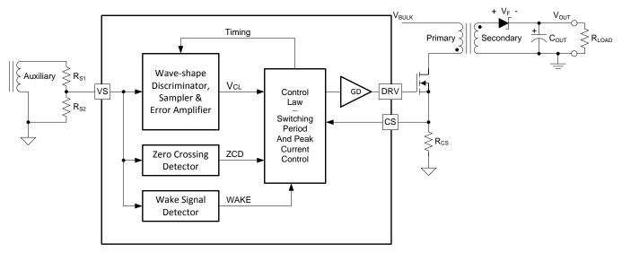
図 13. Simplified Flyback Convertor (with the main voltage regulation blocks)
