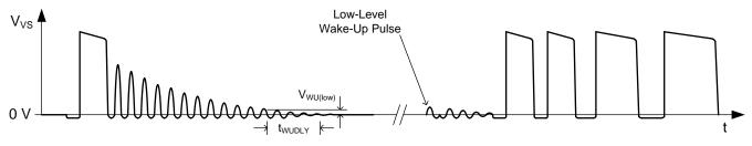
20. Wake-Up Qualification Criteria and Wake-Up Response with Low Wake-Up Signal
