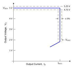
図 18. Typical Output V-I Target Characteristic
