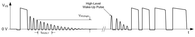
21. Wake-Up Qualification Criteria and Wake-Up Response with High Wake-Up Signal
