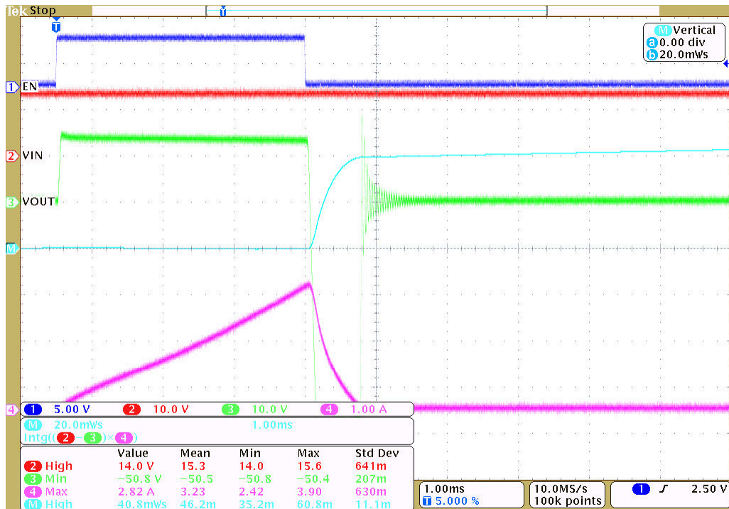
Figure 8-7. Inductive Load Switching-Off Waveform of 40mJ
