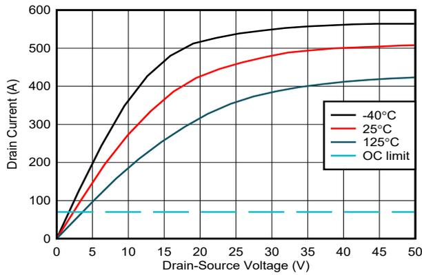
5-5. Drain Current vs Drain-Source Voltage
