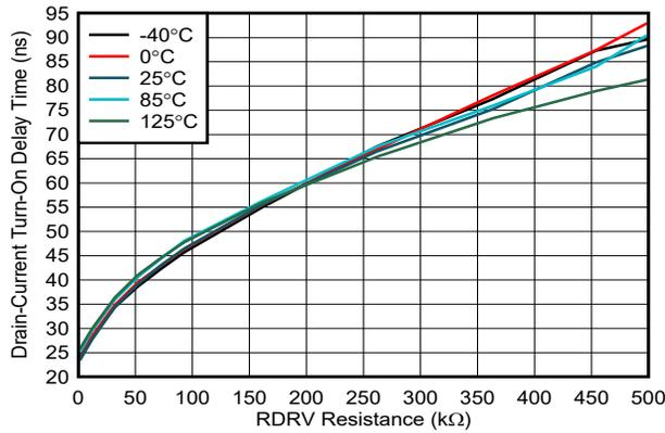
5-1. Drain-Current Turn-On Delay Time vs Drive-Strength Resistance
