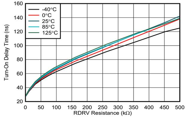
5-2. Turn-On Delay Time vs Drive-Strength Resistance
