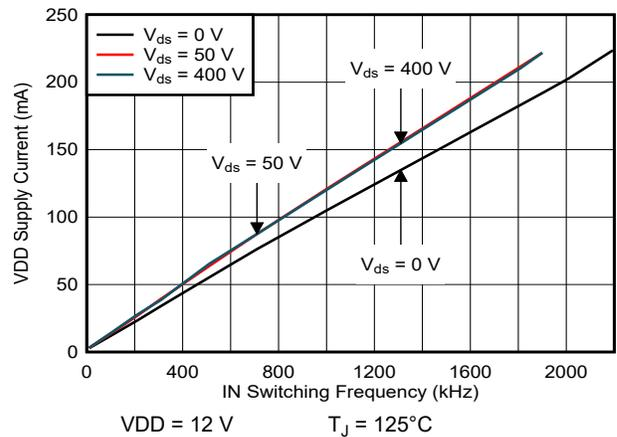
图 5-10. VDD Supply Current vs IN Switching Frequency
