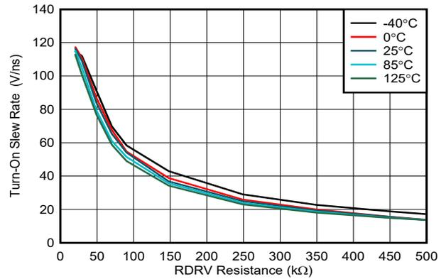
5-4. Turn-On Slew Rate vs Drive-Strength Resistance
