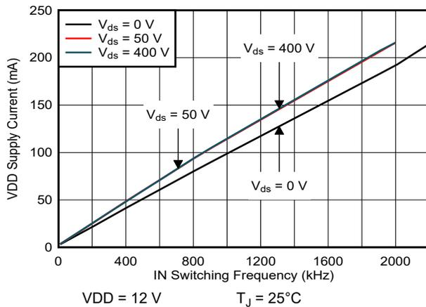
图 5-9. VDD Supply Current vs IN Switching Frequency
