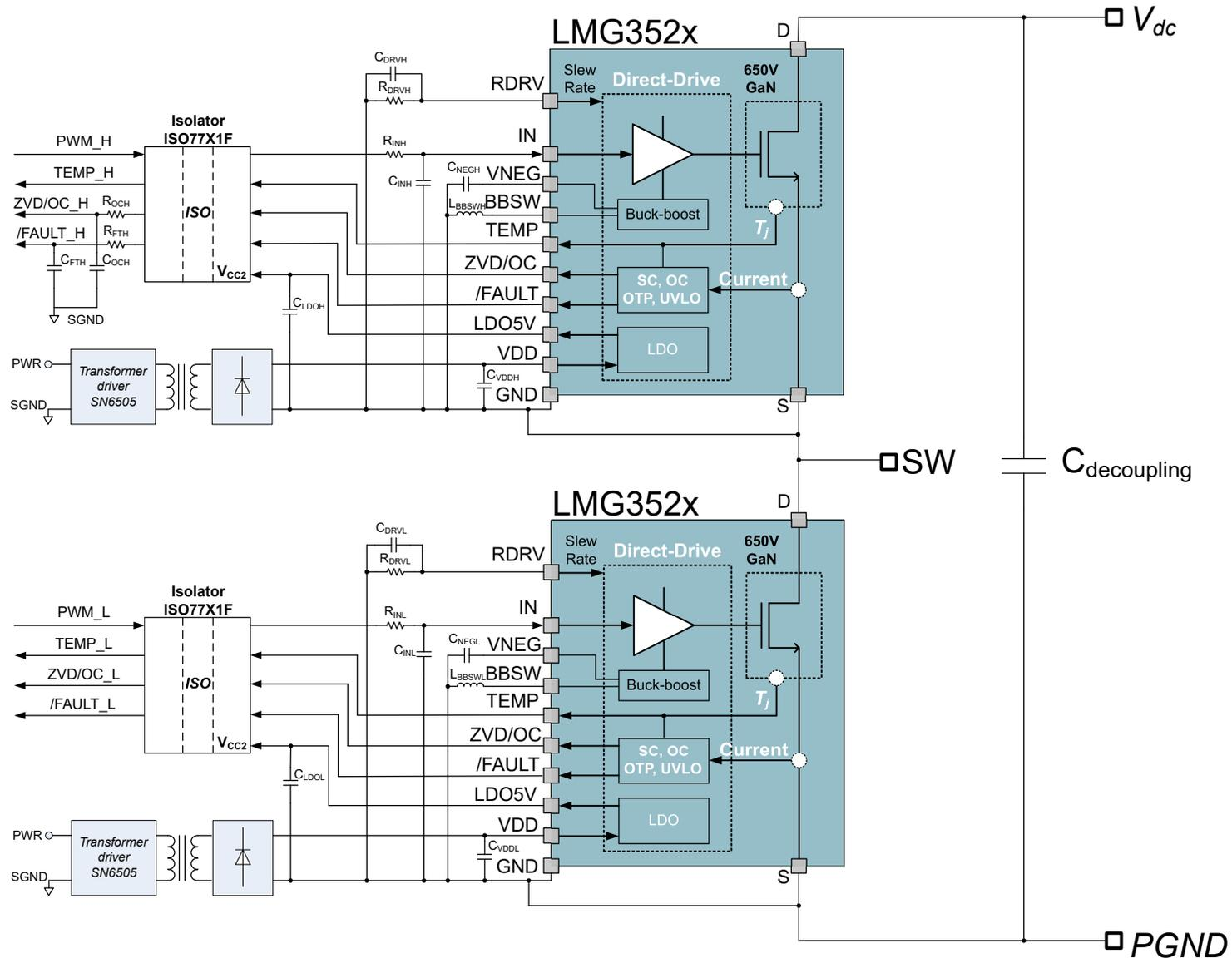
図 8-1. Typical Half-Bridge Application With Isolated Power Supply
