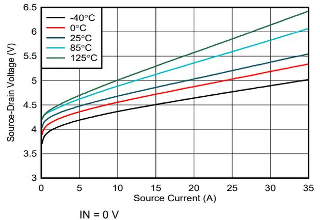
5-6. Off-State Source-Drain Voltage vs Source Current
