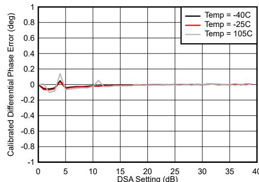
$$\text{微分位相誤差} = \text{Phase}_{\text{OUT}}(\text{DSA 設定} - 1) - \text{Phase}_{\text{OUT}}(\text{DSA 設定})$$
