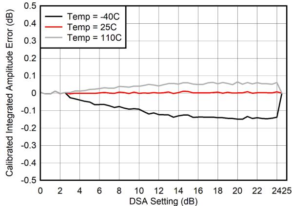
$$\text{積分振幅誤差} = P_{\text{IN}}(\text{DSA 設定}) - P_{\text{IN}}(\text{DSA 設定} = 0) + (\text{DSA 設定})$$
