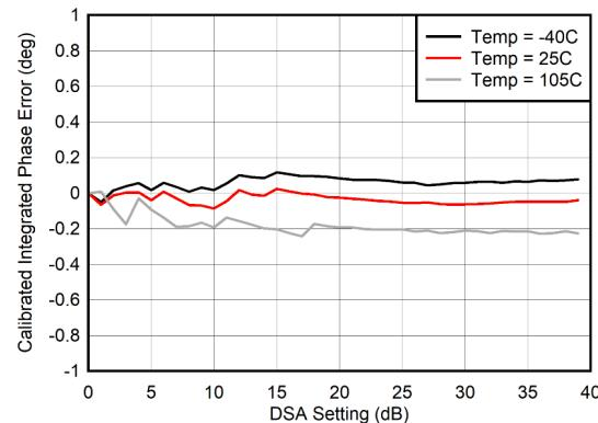
積分位相誤差 =  $\text{Phase}_{\text{OUT}}(\text{DSA} \text{ 設定}) - \text{Phase}_{\text{OUT}}(\text{DSA} \text{ 設定} = 0)$
