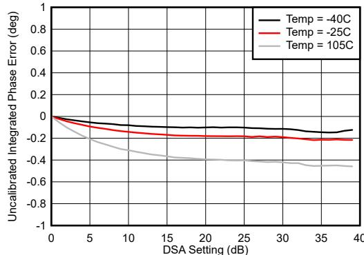
積分位相誤差 =  $\text{Phase}_{\text{OUT}}(\text{DSA 設定}) - \text{Phase}_{\text{OUT}}(\text{DSA 設定} = 0)$
