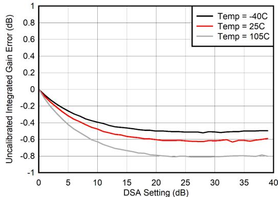
積分ゲイン誤差 =  $P_{\text{OUT}}(\text{DSA 設定}) - P_{\text{OUT}}(\text{DSA 設定} = 0) + (\text{DSA 設定})$
