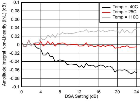
積分振幅誤差 =  $P_{\text{IN}}(\text{DSA 設定}) - P_{\text{IN}}(\text{DSA 設定} = 0) + (\text{DSA 設定})$
