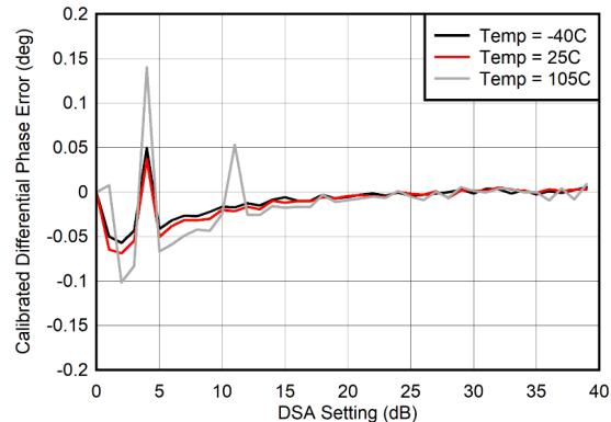
微分位相誤差 =  $\text{Phase}_{\text{OUT}}(\text{DSA 設定} - 1) - \text{Phase}_{\text{OUT}}(\text{DSA 設定})$
