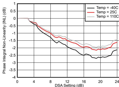
積分位相誤差 =  $\text{Phase}(\text{DSA 設定}) - \text{Phase}(\text{DSA 設定} = 0)$
