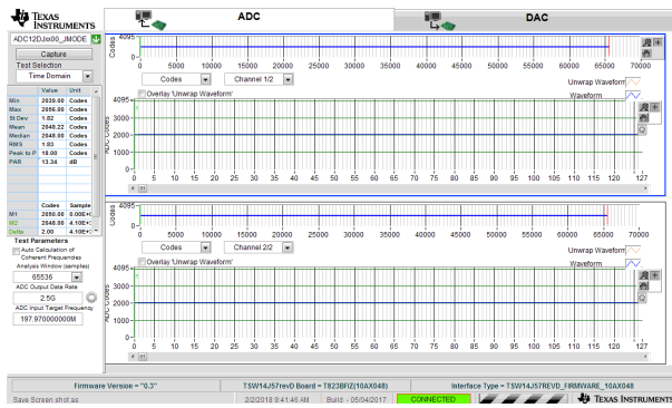
図 7-10. Idle-Channel Noise (No Input) for 2.5-GSPS, Dual-Channel Oscilloscope
