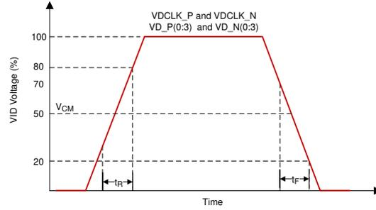
图 6-5. SubLVDS Input Rise and Fall Slew Rate
