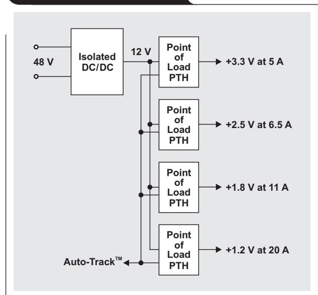
voltages due to features such as TI's Auto-Track™. The only drawback of this architecture is reduced efficiency due to the double conversion required for each voltage.
