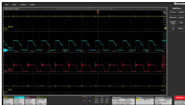
图 3-34. Vin = 90Vac , Vout = 12V
