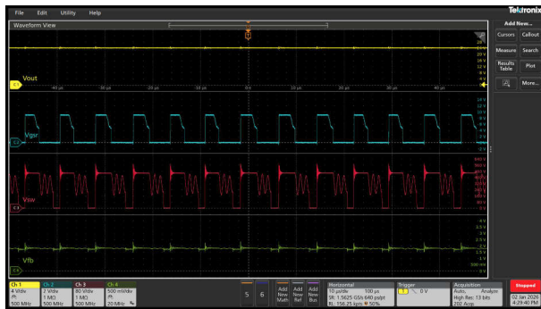
图 3-32. Vin = 230Vac , Vout = 24V
