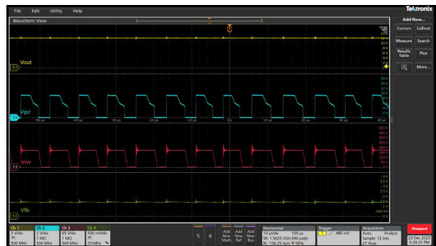
图 3-35. Vin = 115Vac , Vout = 12V
