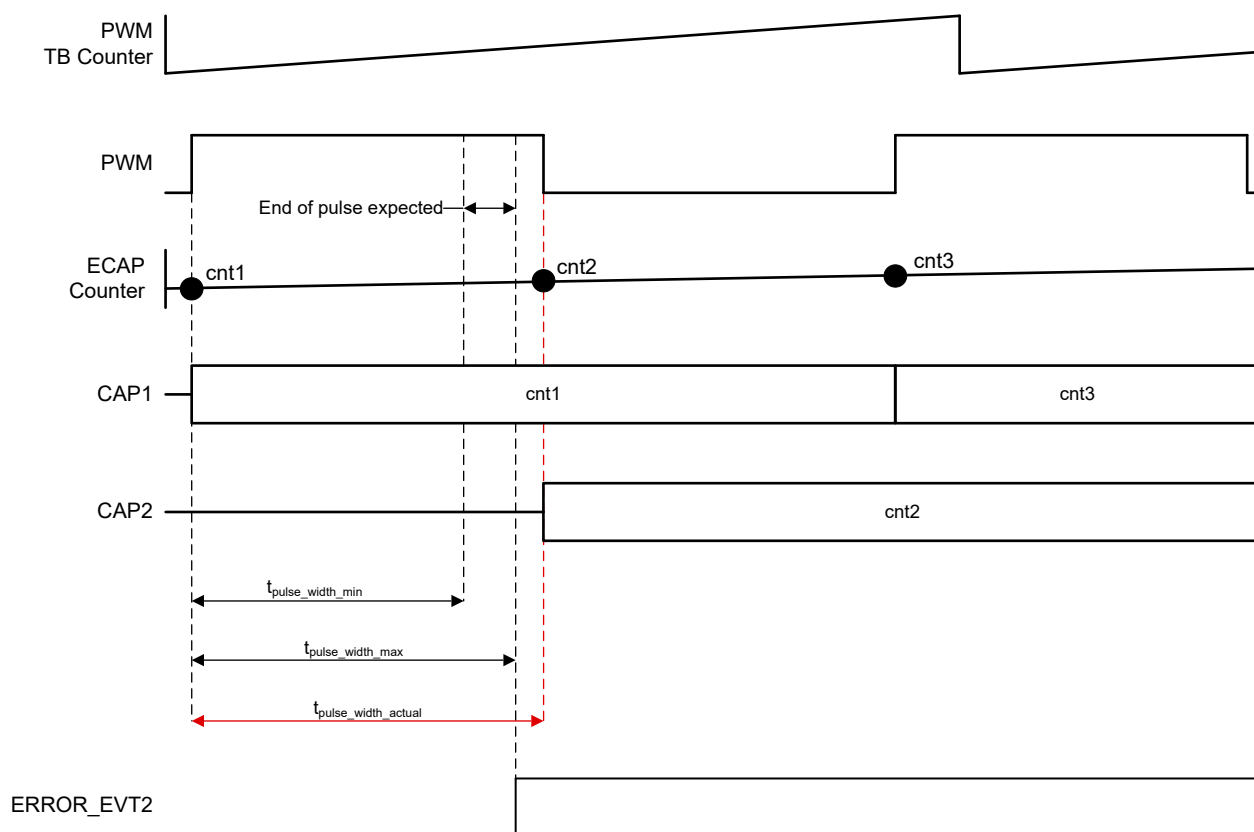
Figure 25-12. ECAP Signal Monitoring Unit Pulse Width Error Example
