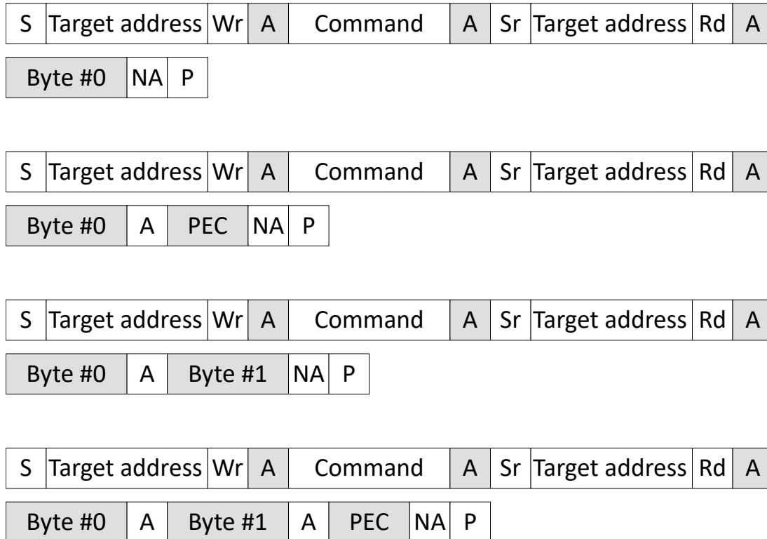
Figure 34-19. Read Byte and Read Word Messages With and Without PEC
