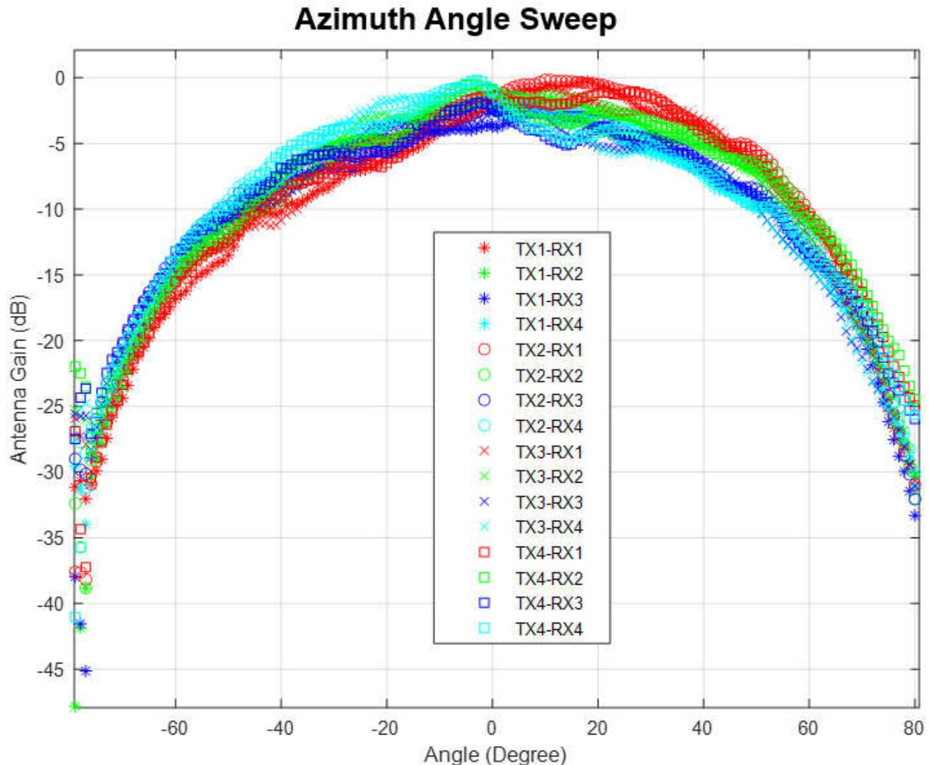
Figure 2-19. Azimuth Radiation Pattern
