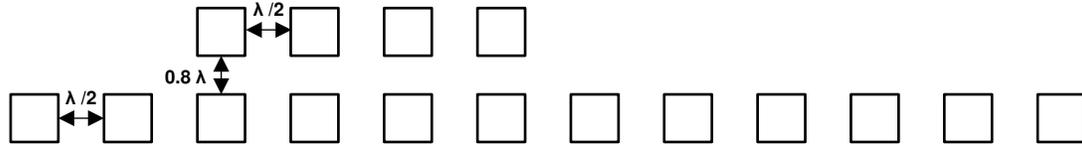
Figure 2-18. Virtual Antenna Array
