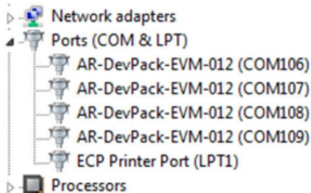
**Figure 2-24. Installed FTDI Drivers**
