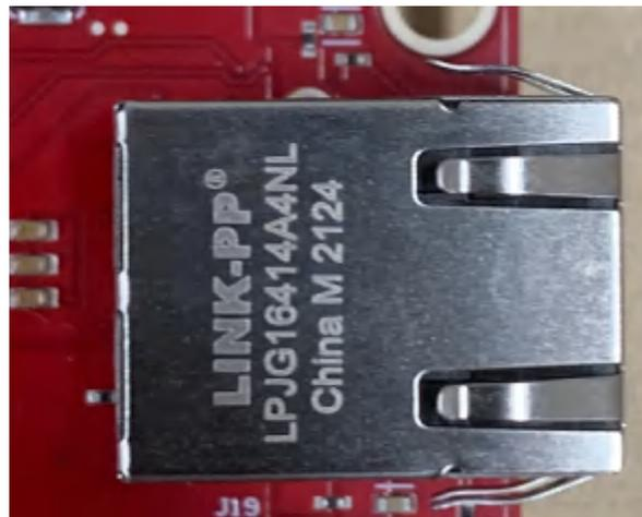
**Figure 2-12. RJ45 Connector**
