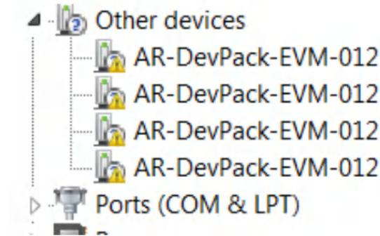
**Figure 2-23. Uninstalled FTDI Drivers**
