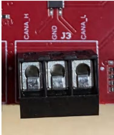
**Figure 2-10. CAN\_A Connector**
