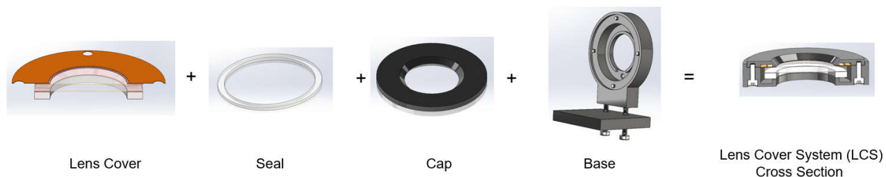
Figure 3-5. Flat Lens LCS (LCS): Lens Cover + Cap + Seal + Base
