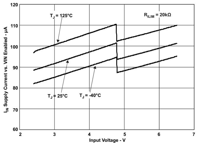
Figure 13.  $I_{IN}$  – Supply Current, Output Enabled –  $\mu A$
