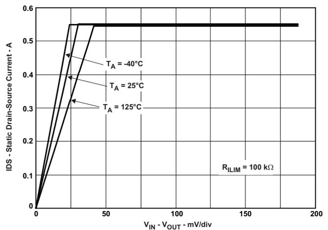
Figure 15. Switch Current Vs. Drain-Source Voltage Across Switch
