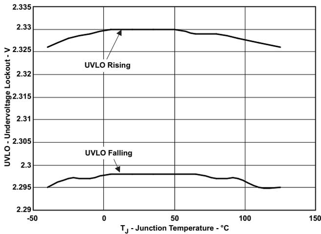
Figure 10. UVLO – Undervoltage Lockout – V
