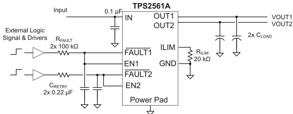
Figure 20. Auto-Retry Functionality With External EN Signal
