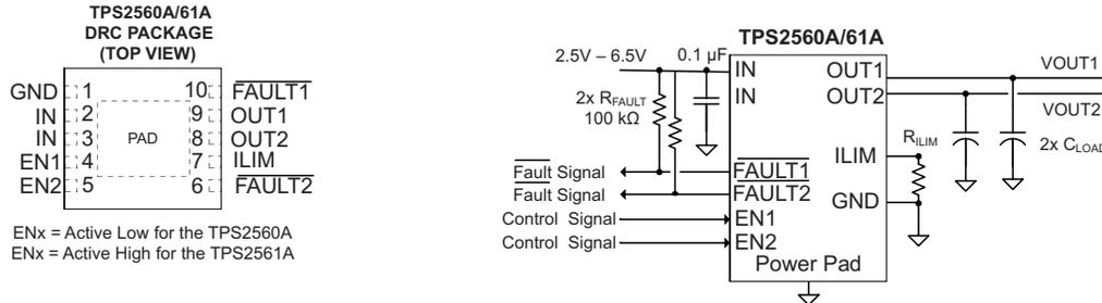
Figure 1. Typical Application as USB Power Switch
