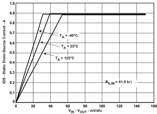
Figure 16. Switch Current Vs. Drain-Source Voltage Across Switch
