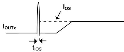
Figure 3. Response Time to Short Circuit Waveform
