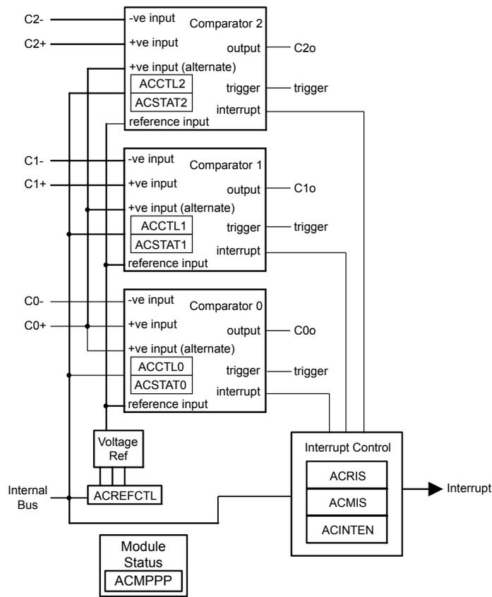
**Note:** This block diagram depicts the maximum number of analog comparators and comparator outputs for the family of microcontrollers; the number for this specific device may vary. See page 1228 for what is included on this device.
