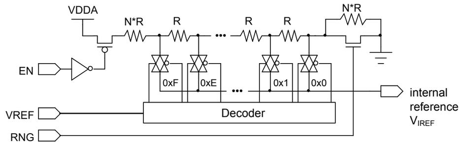
**Note:** In the figure above,  $N \cdot R$  represents a multiple of the  $R$  value that produces the results specified in Table 19-2 on page 1217.
