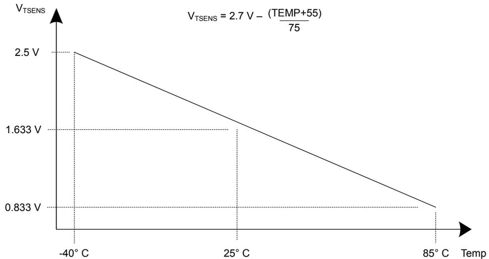
The temperature sensor reading can be sampled in a sample sequence by setting the  $TS_n$  bit in the **ADCSSCTLn** register. The temperature reading from the temperature sensor can also be given as a function of the ADC value. The following formula calculates temperature (TEMP in  $^{\circ}C$ ) based on the ADC reading ( $ADC_{CODE}$ , given as an unsigned decimal number from 0 to 4095) and the maximum ADC voltage range ( $V_{REFP} - V_{REFN}$ ):
