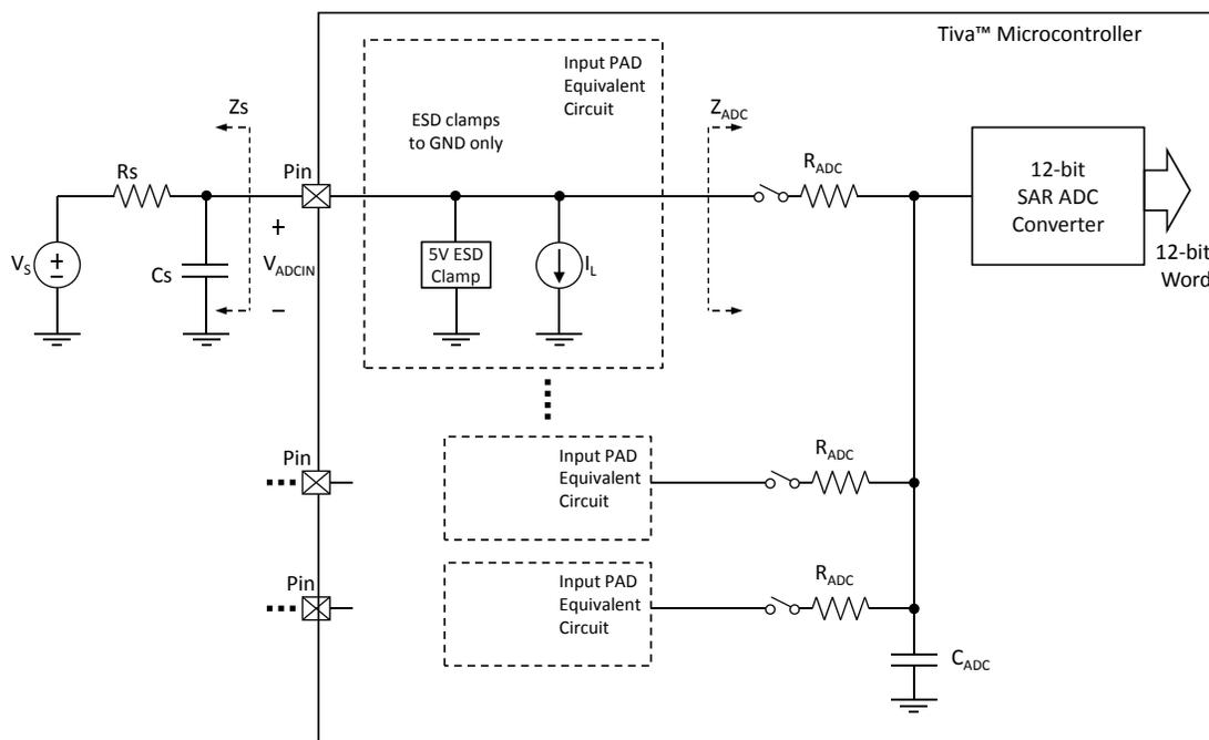
The ADC operates from both the 3.3-V analog and 1.2-V digital power supplies. The ADC clock can be configured to reduce power consumption when ADC conversions are not required (see “System Control” on page 227). The analog inputs are connected to the ADC through specially balanced input paths to minimize the distortion and cross-talk on the inputs. Detailed information on the ADC power supplies and analog inputs can be found in “Analog-to-Digital Converter (ADC)” on page 1388.
