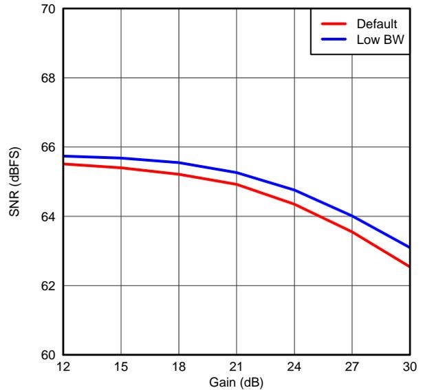
**Figure 10. SIGNAL-TO-NOISE RATIO vs GAIN ACROSS BANDWIDTH MODE**
