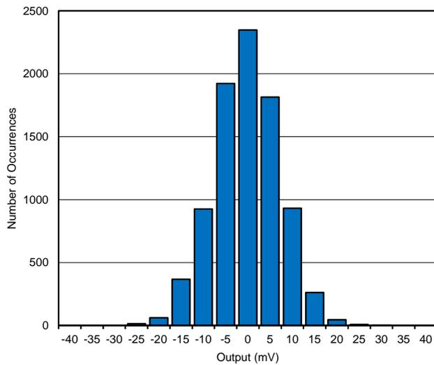
Figure 3. OUTPUT OFFSET HISTOGRAM (Gain = 30 dB)
