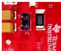
Figure 2-13. Current Measurement Point
